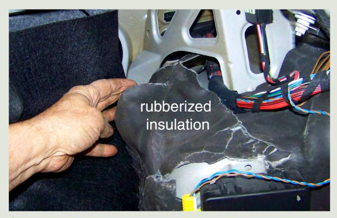
Open the trunk. Pull back the inner liners. Then pull back the rubberized insulation covering the upper shock mounts. (Be warned that this rubberized material may crumble from age when it is moved.)
