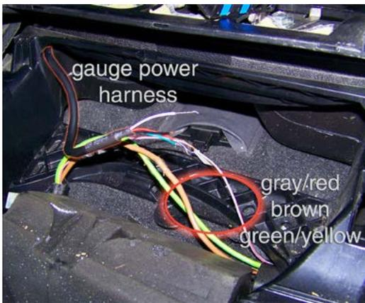
Removing the center console cover exposes the brown, green/yellow, and gray/red wires that provide ground and power to the gauge harness.
