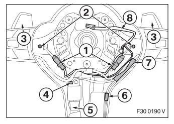
Loosen and remove the screw (1) on the back of the steering wheel (2).
