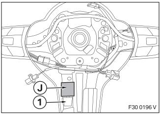
Do not crush or trap the cables. ◀
