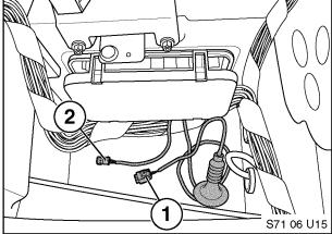
Note: Vehicles with optional Comfort Access (1) and/or PDC (2) will have one or both body access holes occupied. Vehicles without either option will have a blank plug covering these holes.
