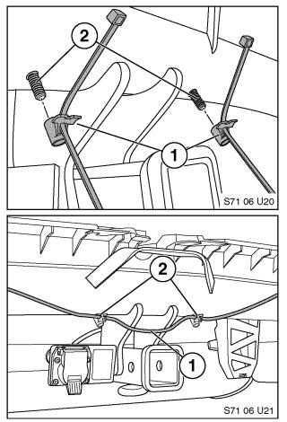
1. Install wire-ties with brackets (1) from installation kit onto mounting studs (2), located on trailer hitch cross member, as illustrated.
