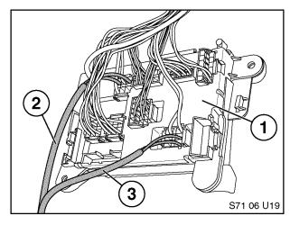
17. Connect trailer wiring harness ground (single brown wire with ring connector) (1) to vehicle ground point as illustrated.
