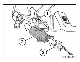
When towing a trailer with a four-pin wiring harness (3). Use the 4-pin to 7-pin adaptor (2) included in the installation kit to connect the trailer electrical system to vehicle connector (1).
