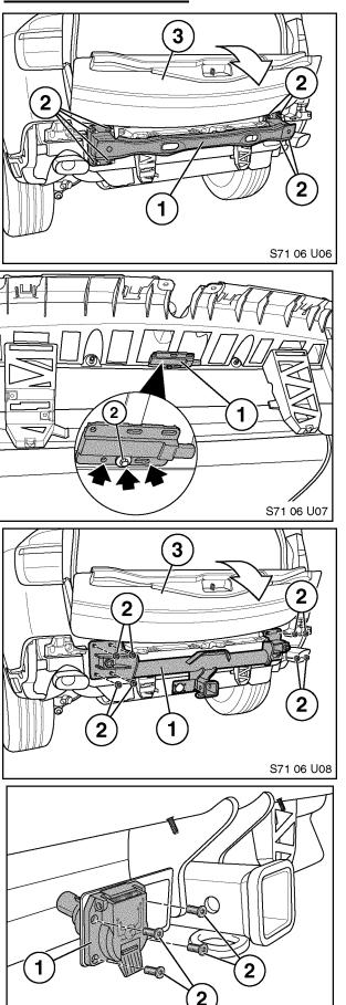
1. Remove and discard steel bumper (1) and eight mounting nuts (2) from vehicle.
