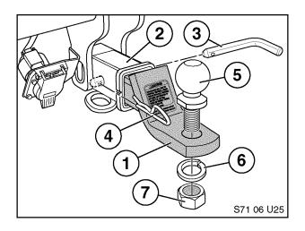
Install trailer ball (5) onto ball mount (1) with lock washer (6) and nut (7).
