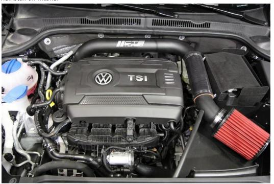
Start and test drive vehicle. Check for proper operation and any vacuum/boost leaks.
