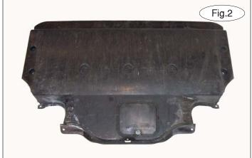
1. Remove 10 Philips fasteners and two 10mm (head) bolts attaching the factory rear skid plate to the subframe. The pieces should be removed as shown in Figures 1 and 2.
