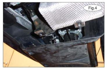
2. Using a pair of pliers, remove all the slip nuts from the mounting points on the subframe. Figure 3 shows the location of two of the front mounting points. Replace these slip nuts with the 12 supplied 5/16-18 slip nuts. Figure 4 shows two of the front mounting points with the new slip nuts installed.
