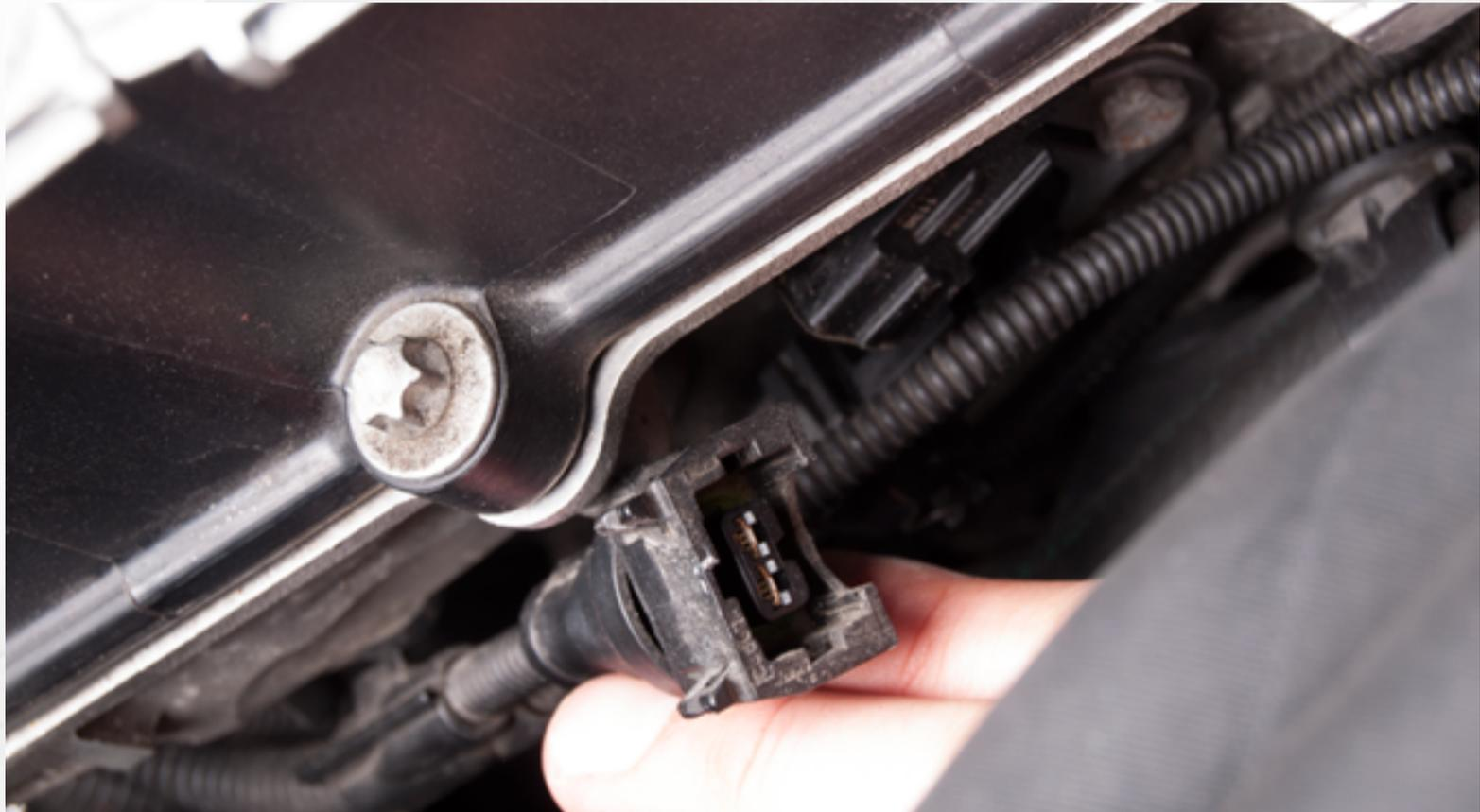
We used a hinged socket wrench to easily remove the two bolts holding the solenoids in place. Whichever tool you choose, it should positively engage with the bolt to avoid stripping - you will be reusing them.
