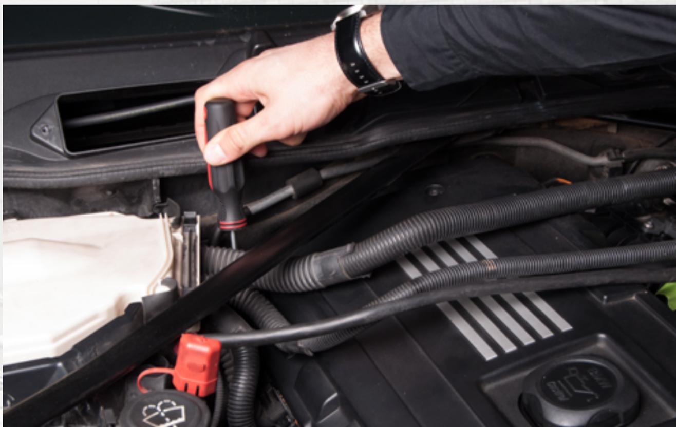
Depending on the manufacture date and options installed on your vehicle, you may notice oil cooler hoses in the front of the cylinder head. Removing or repositioning the oil cooler and hoses may make the project easier.
