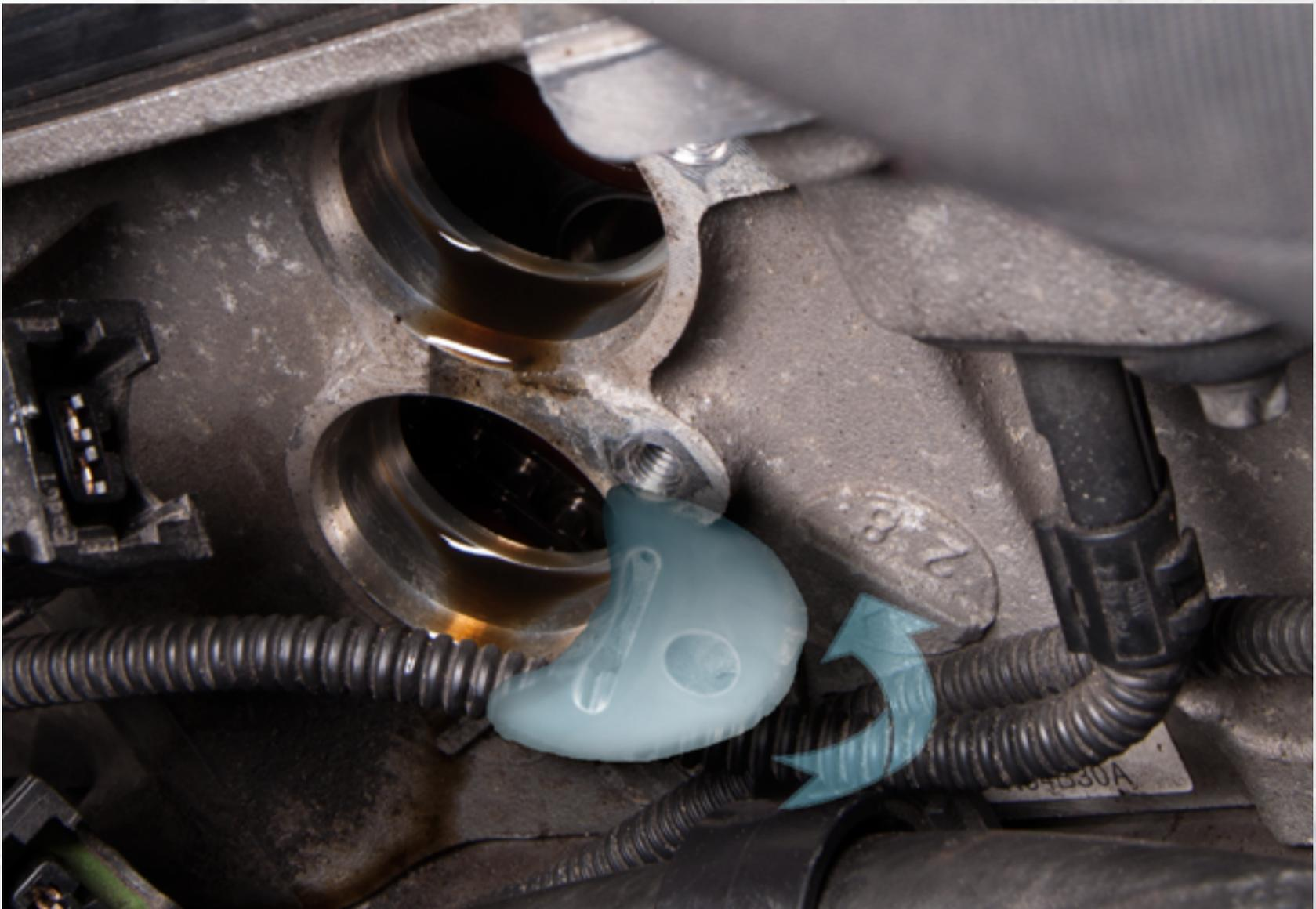
Orientation of solenoid mounting bracket before installation shown above. Turn solenoid counter-clockwise until the bolt is aligned with the hole and the solenoid is fully inserted.
