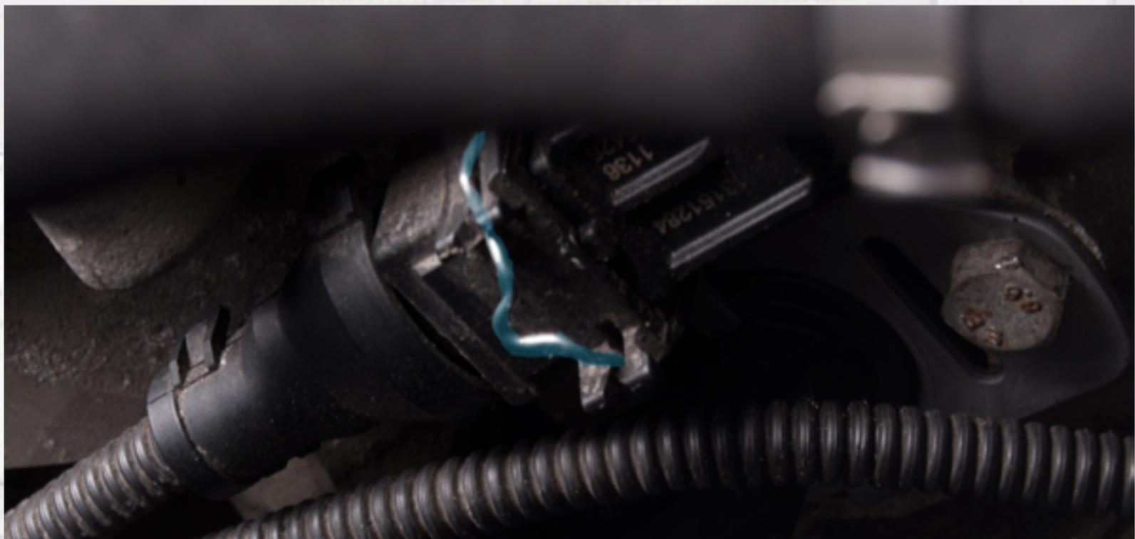
With the electrical harnesses removed, you must now decide what type of tool will place the 10mm socket on the bolt head while giving you room and leverage to torque it free.
