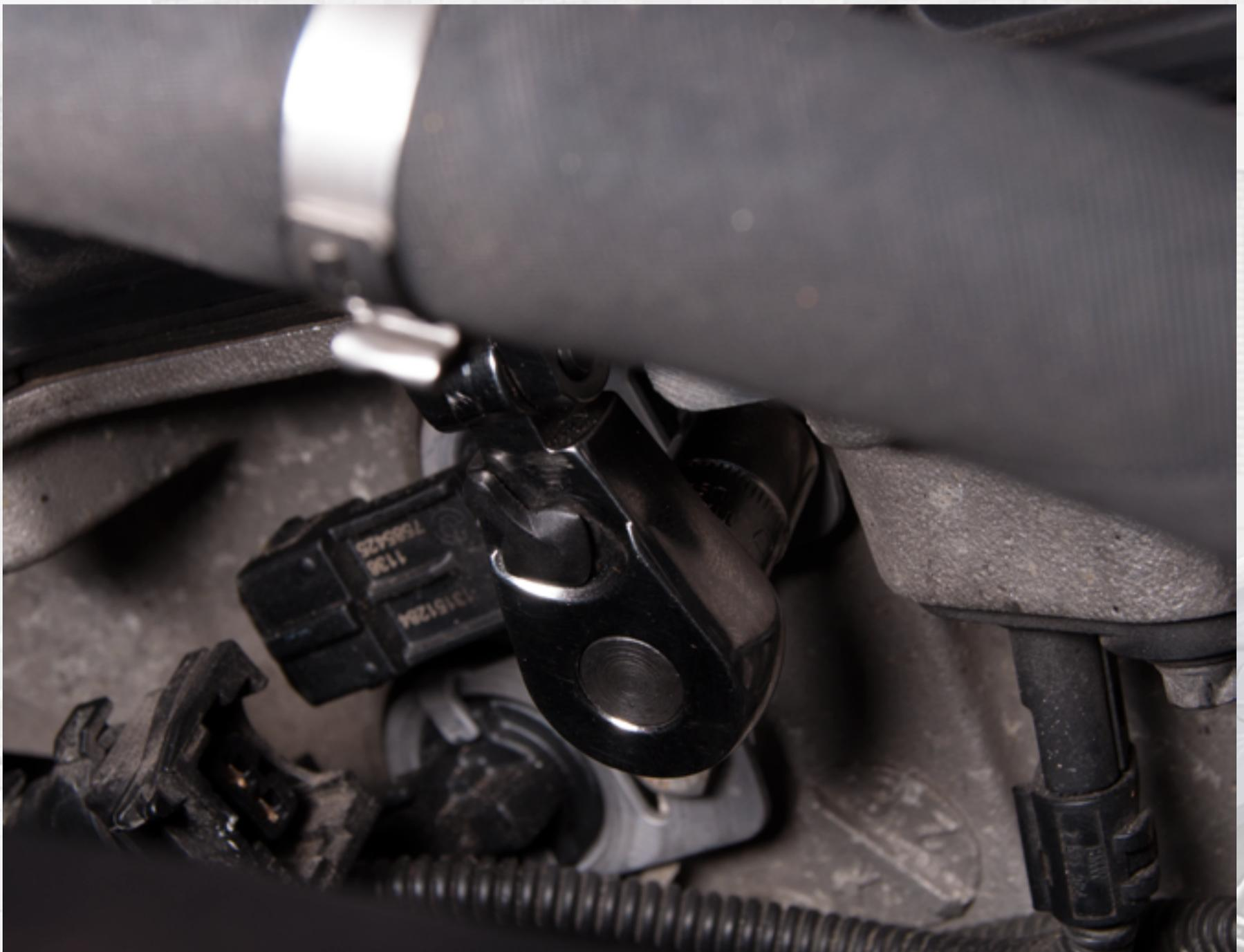
Before removing the valve itself, you may want to place a rag underneath the valve opening you will be exposing - VANOS is an oil routing mechanism; there may be some oil leakage.
