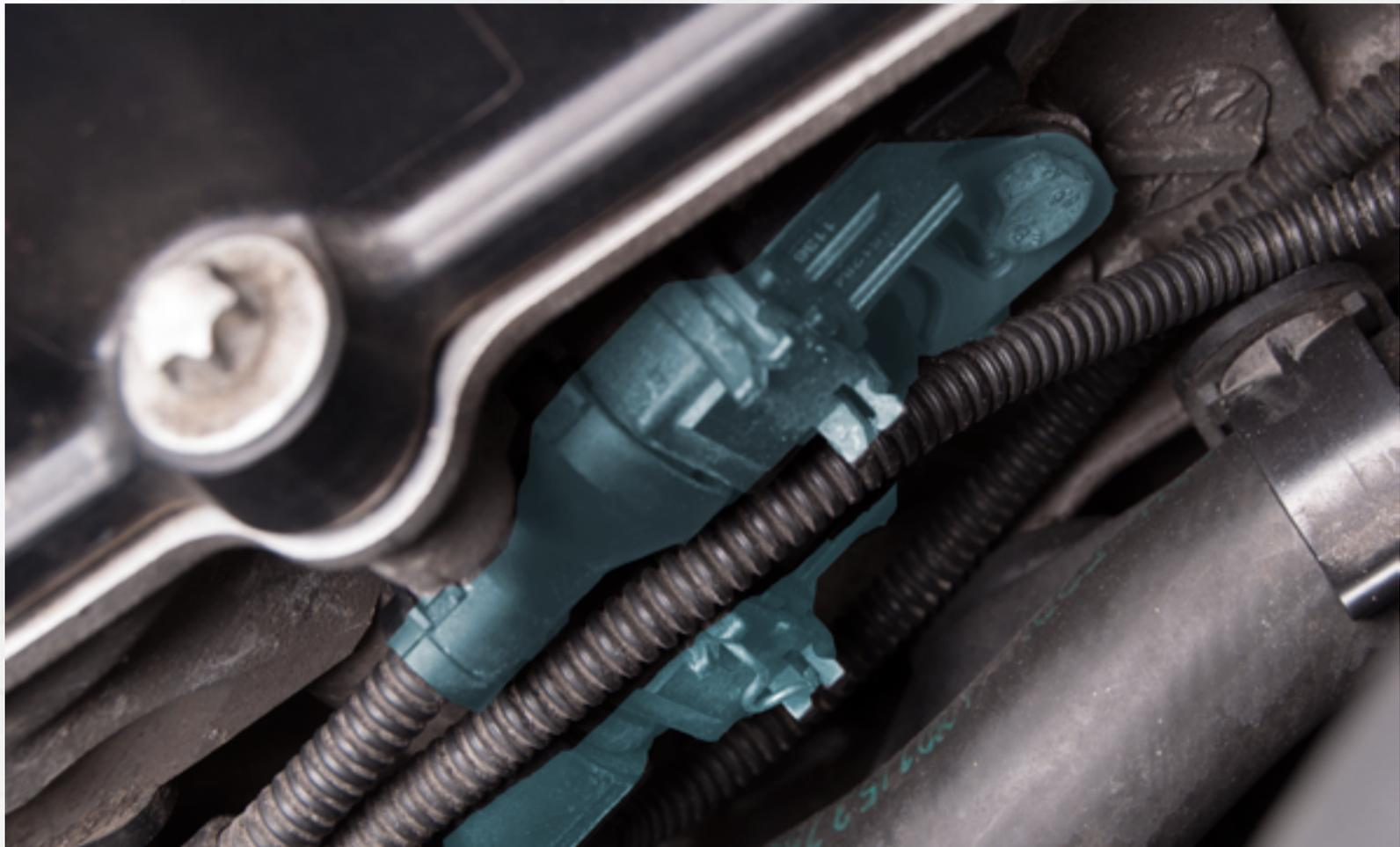
A metal clip secures the electrical connection to the solenoid. Press it in while pulling the connector out away from the solenoid.
