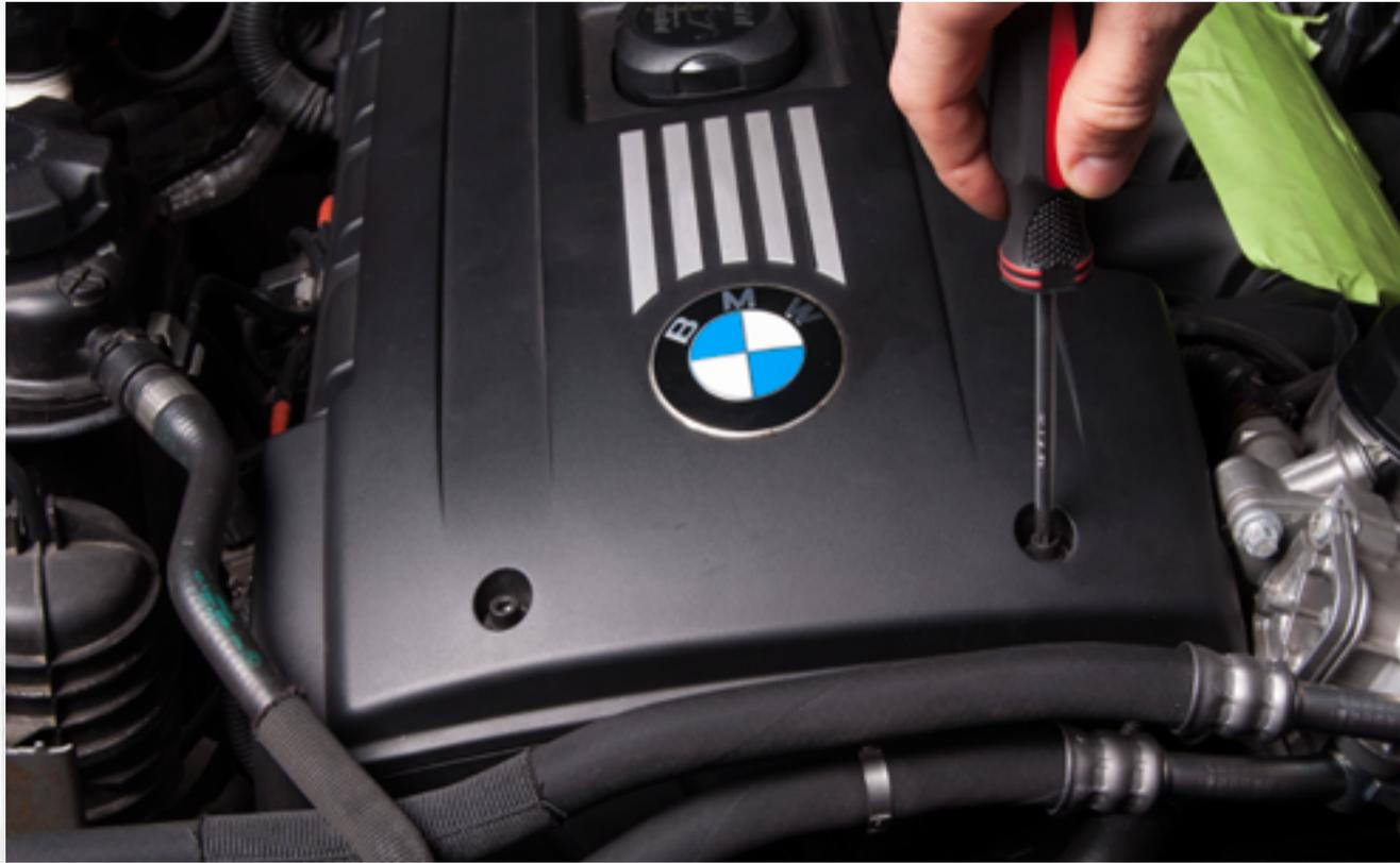
It is not necessary to fully remove the screws from the recesses in order to lift the engine cover out of the engine bay.
