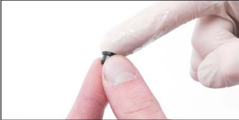
1. Lubricate the new grommet seal with brake fluid.
