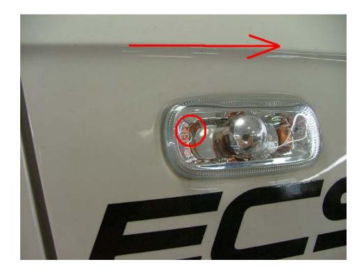
To remove the OEM fender markers, slide the light forward. While holding it forward, pull on the corner of the marker marked E1, the whole assembly will release its self from the fender.
