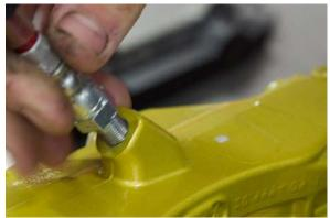
Tighten the brake line using a 14 mm box wrench. Exercise caution and be attentive not to over tighten the brake line.
