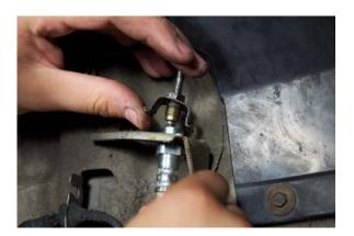
When tightened, the brake line will look like the picture to the right.
