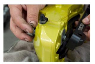
The next step is to install the brake line. Remove the rubber cap from the caliper and start threading in the new line.
