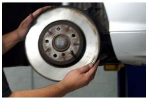
It is recommended that you thoroughly clean the mounting surface where the new rotor will sit to ensure there is no corrosion where you mount the rotor.
