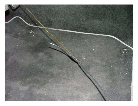
Tape the long control wire to the end of the hanger inside the vehicle. Proceed to carefully pull it through the firewall in a manner that will not bend the fragile female pin ends crimped on the wire.
