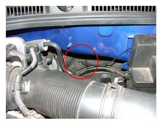
With the wire completely pulled through, a thin slice in the grommet will ensure the wire does not rub on the fire wall.
