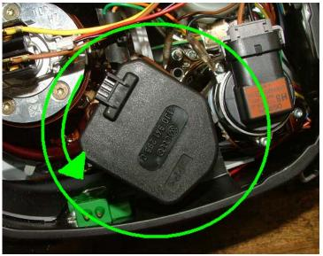
Twist motor assembly in direction of arrow to install.
