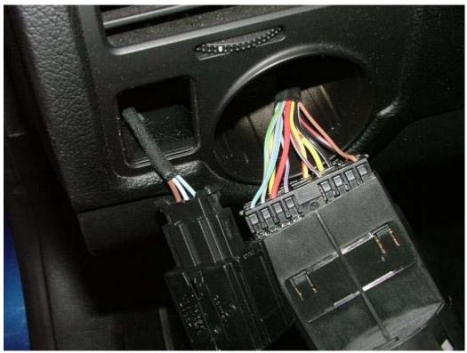
With the headlamp switch removed, hook your finger through the headlamp switch recess and push on the back of the dimmer switch until it pops out of its slot. Unclip the dimmer switch from the harness.
