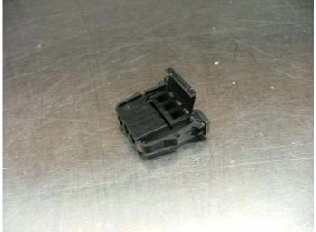
Take a small screwdriver and as indicated in the above diagram, pry the pin lock up to release the dimmer control wires.
