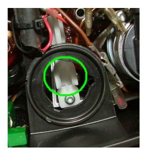
The ball on the end of the leveling motor post must be inserted inside the circled plastic groove.
