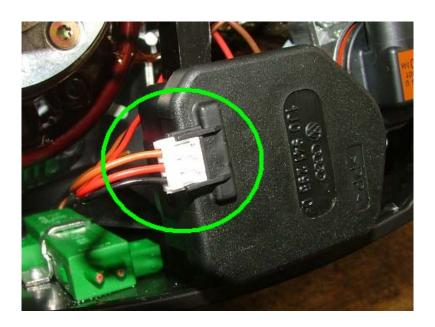
Clip loose 3 wire connector on, and repeat procedure for the other headlight assembly.
