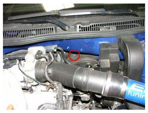
Remove the above grommet and insert a straightened coat hanger or similar device through this hole.
