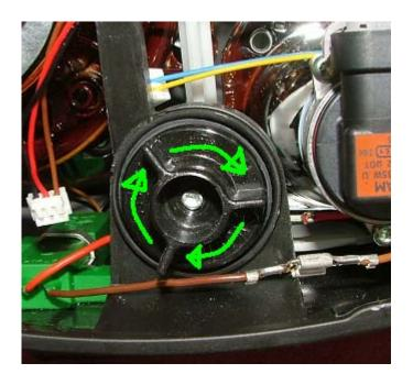
Start by removing the "dummy" holder post from the headlight. The "dummy" must be twisted toward the right to remove.
