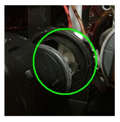
Ensure the ball is seated in the groove before completely installing the motor.
