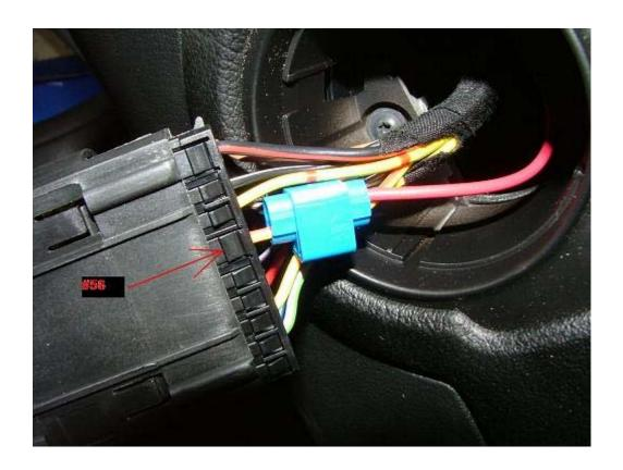
Using the supplied scotch lock, connect the red wire from the rheostat to the yellow / red wire (#56) on the headlamp connector. This is the power wire for the rheostat leveling control signal
