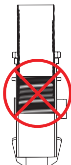
Not OK, threads are showing.
