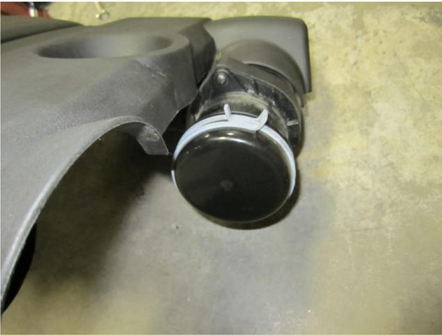
k) Install the cap (8-209) onto the engine cover and secure with the pressure clamp that was released in 2b.
