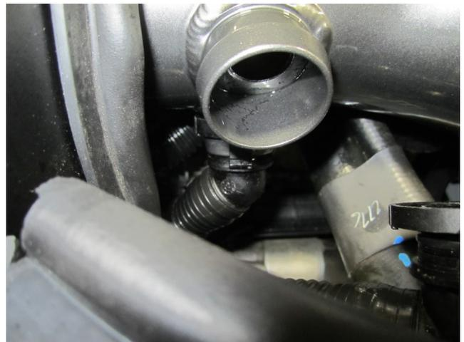
f) Before installing the tube into the hose at the throttle body, make sure to connect the lower (smaller) air injection connector onto the AEM tube. **Note: Using warm soapy water on the O-ring (located in the connector) will help ease the connector onto the tube fitting. For models that do not have the larger connector, use the supplied cap to cap off the vent on the intake tube.**
