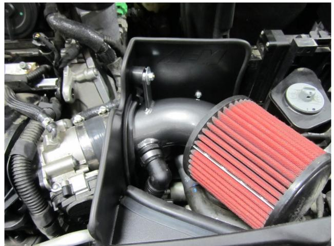
j) Install and tighten the air filter and hose clamp (9452) onto the AEM intake tube. **Note: Rotate the filter for best clearance, so it does not make contact with anything in the engine compartment.**
