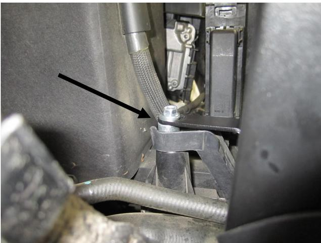
e) Using the supplied hardware, install the bolt, washer and spacer (1-1016 & 08275 & 07849) to attach the bracket to the post where the bolt was removed in 2f.
