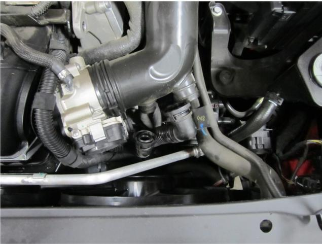
e) Release the pressure on the clamp at the throttle body and remove the stock intake tube. **Note: Do not discard any of your stock intake.**
