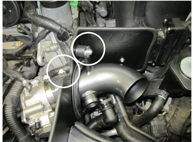
h) Install and tighten the washer and nut onto the mount (08160 & 444.460.04). Then make sure the AEM tube is fully seated in the hose on the throttle body and tighten the hose clamp.
