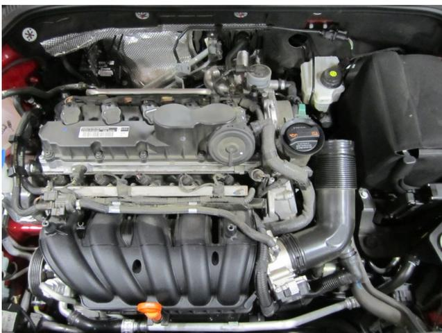
c) Remove the engine cover from the vehicle.
