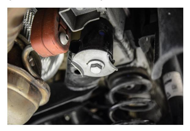
**Step 3** – Once the subframe bolt is removed, use a small pry bar to separate the factory washer from the rubber bushing.
