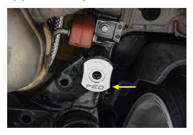
**Step 6** – Install subframe bolt using an 18mm Socket. **Note:** We recommend replacing the original subframe bolts with new pieces, as they are stretch bolts that are intended for a one-time use. **If you opt to reuse the stock bolts, torque them to 90 Nm with Blue Loctite.**
