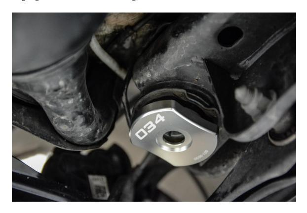
**Step 12** – Install subframe bolt using an 18mm Socket. **Note:** We recommend replacing the original subframe bolts with new pieces, as they are stretch bolts that are intended for a one-time use. **If you opt to reuse the stock bolts, torque them to 90 Nm with Blue Loctite.**
