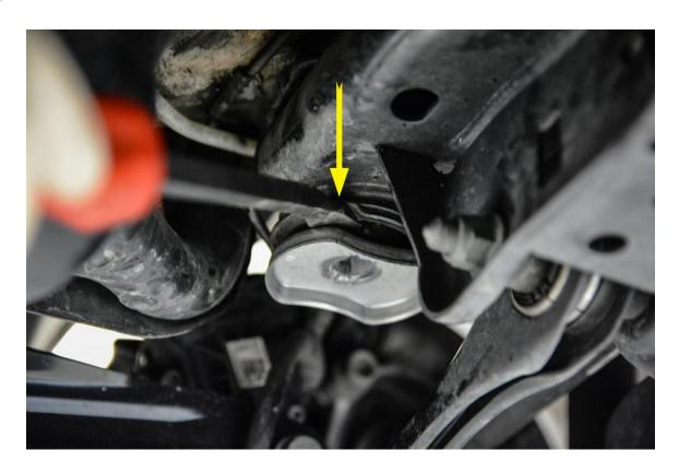
**Step 10** – Align the front-specific 034Motorsport Rear Subframe Insert (601-0030) with the voids in the factory rubber bushing.
