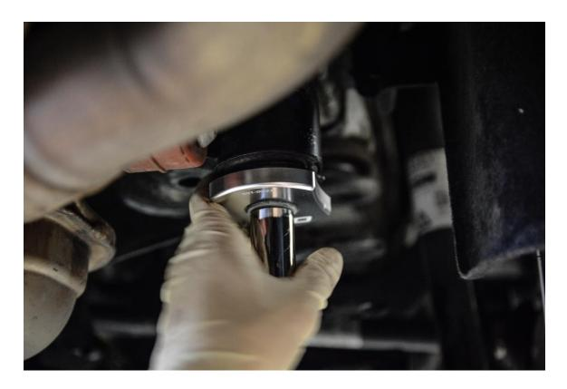
**Step 7** – Torque subframe bolt to 90 Nm + 90° Turn. (Arrows point toward the front of the car for reference)
