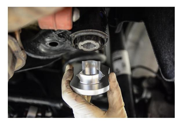
**Step 5** – Install rear subframe insert by pressing into the rubber voids of the factory rubber subframe bushing. We recommend aligning the insert such that the 034 logo is toward the front of the car.
