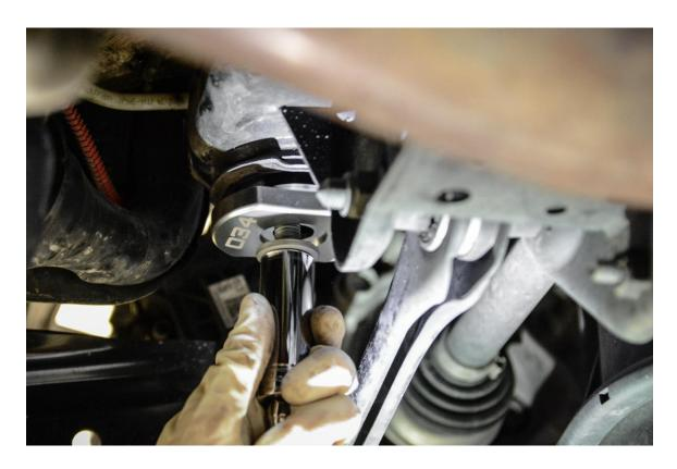
**Step 13** – Torque subframe bolt to 90 Nm + 90° Turn. (Arrows point toward the front of the car for reference)
