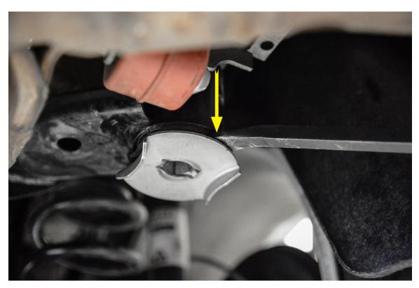
**Step 4** –Align the rear-specific 034Motorsport Rear Subframe Insert (601-0031) with the voids in the factory subframe bushing.
