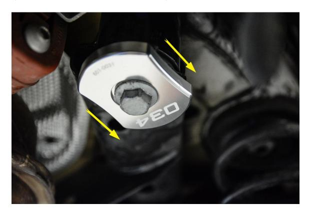
**Step 8** – Using an 18mm Socket, remove the front bolt securing the rear subframe to the chassis.
