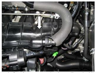
At the front (transverse engines) you will see the OEM vacuum hose connector. By squeezing the sides of the OEM connector the locating clips are released so that the connector can be withdrawn.
