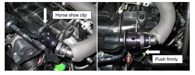
The Forge vacuum take-off adaptor is installed as shown. It is necessary to push the adaptor onto the spigot so that the retaining (horse shoe type) clip can be slid into place fully.
