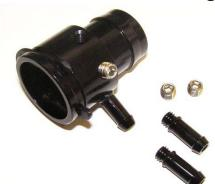
The vacuum tap has 3 tap provisions on it and it is supplied with multiple vacuum nipples and blanking plugs for you to select the number of provisions you will need on your application. It is recommended that all vacuum nipples and port plugs are secured with medium strength semi-permanent Loc-Tite or similar ( not supplied)
