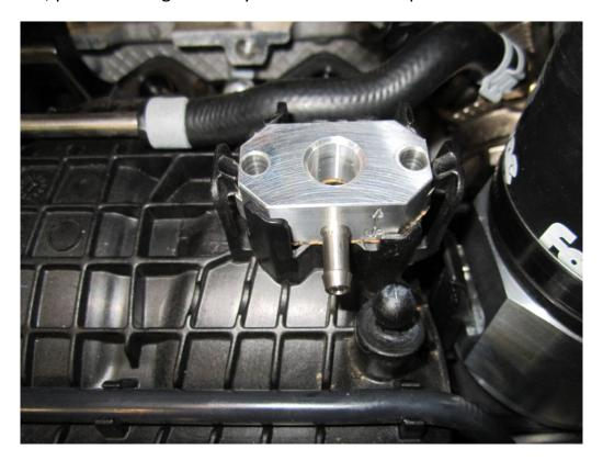
14. Now fit the sensor to the take off block using the posi screws provided and tighten with a posi drive screwdriver.
