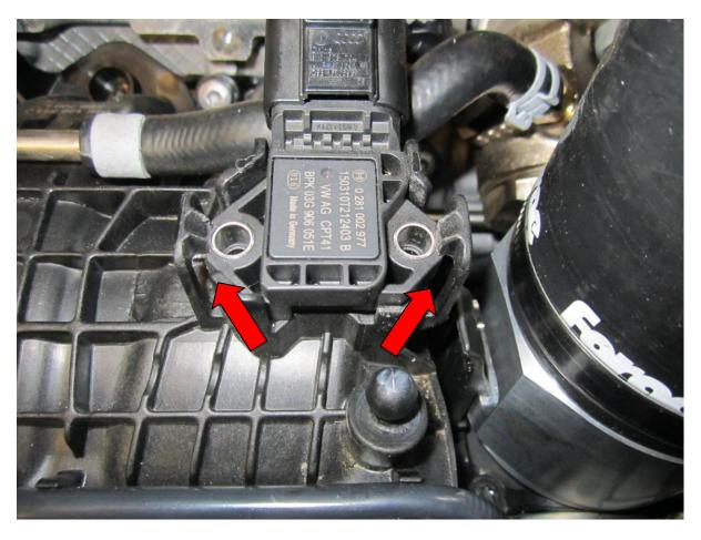
13. The boost source take off adaptor must now be placed in position on the manifold, push down again until you feel it click into position.
