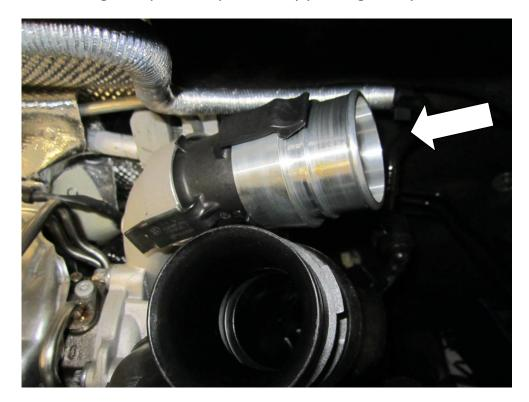
9. You must now remove the OEM o-ring from the boost pipe and place in the new Forge Motorsport throttle body coupler.
