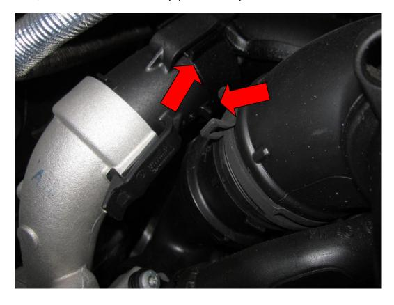
8. Insert the new Forge coupler into position by pushing until you hear it click.
