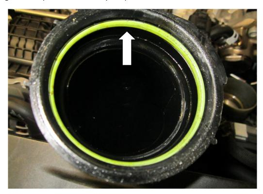
10. Place the o-ring in the new coupler where arrowed below.
