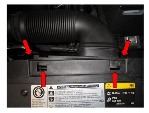
3. Remove the pipe from your airbox to the cam cover breather.
