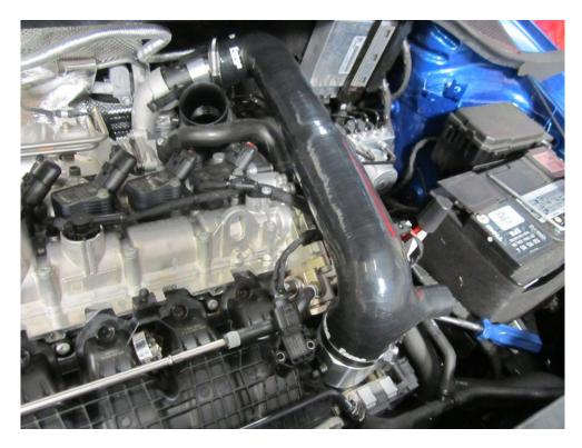
16. Now fit the new Forge Motorsport dump valve into position and tighten the hose clamp that holds it in position.
