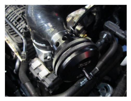
17. Now connect the vacuum pipe supplied from the top of the dump to the boost take off block you fitted in section 14. Using the tie clips provided, fasten the vacuum tube to the coolant pipe pictured and arrowed white.
