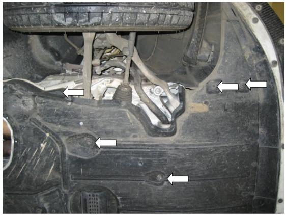
2. Undo the screws securing the strip of plastic under the front edge of the bumper (10 in total) , and remove it from the car.
