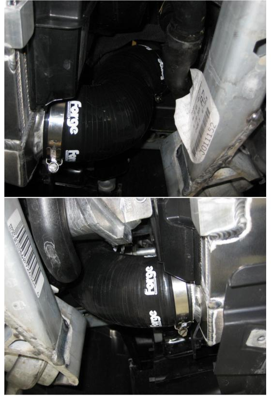
10. The bottom jubilee clips can be easily done up, however the upper clips are very hard and will require a ratchet with a long extension and 7mm socket in order to do up the clips. Use the photos below as a guide as to how to position the ratchet to tighten the clips. Ensure that the clips are square to the hose before tightening.
