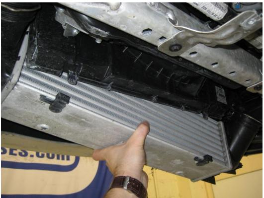
7. Both standard intercooler pipes need to be removed from the car. BMW use a 'use once' clip with a locking joint that needs to be prised apart with a screwdriver, or cut off with a dremel or similar.
