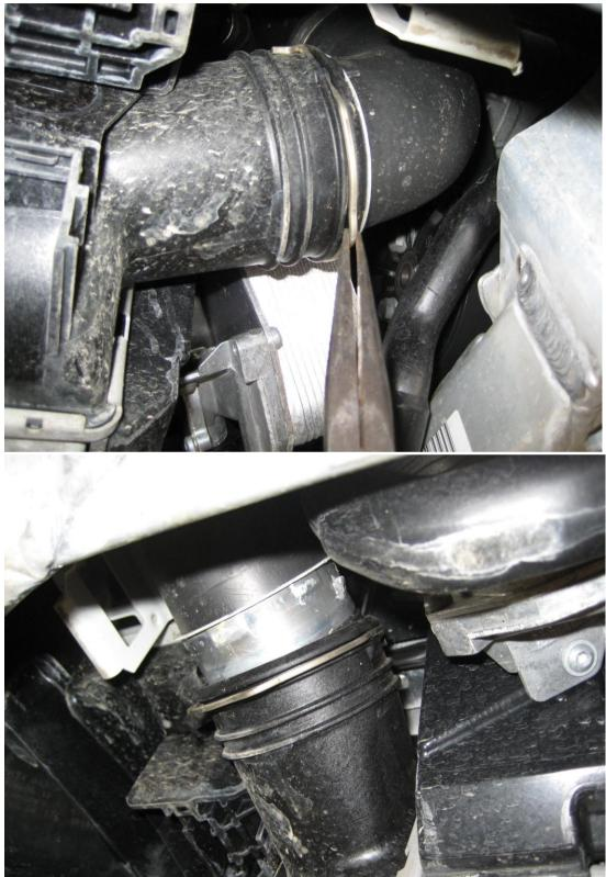
4. Rotate the two clips on the underside of the intercooler to the 'unlocked' position, and remove the plastic piece under the intercooler that they were securing.
