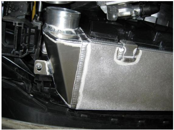
9. The S-shaped bend mounts on the right side of the car (drivers side, UK) and the kinked 90 degree bend mounts on the left side (drivers side, USA and Europe). Use silicon lubricant (dashboard cleaner works well) on the inside of the hoses to help fitting, and add the jubilee clips loosely before fitting the hoses. On the left side, take care when pushing the Forge hose on that you don't push the OEM hose off the clip on the rear edge of the radiator.
