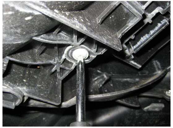
6. Remove the intercooler from the car with care. On the 335 it's necessary to bend back the lower edge of the bumper to facilitate removal. Take care that the clips on the back of the intercooler release from the fan shroud.
