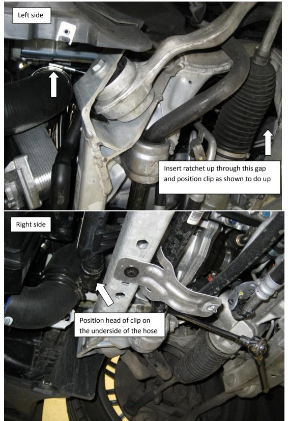
11. Installation is now complete, follow steps 2 and 1 in reverse order to replace the undertrays. The undertray will be a little tighter to fit but will still screw up.
