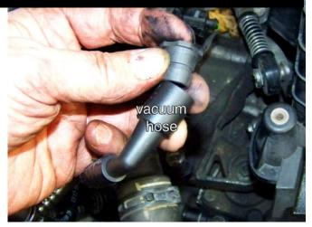
If you start the engine to check for leaks with the air filter housing off the car, expect to throw a MAF sensor DTC that illuminates the MIL.
