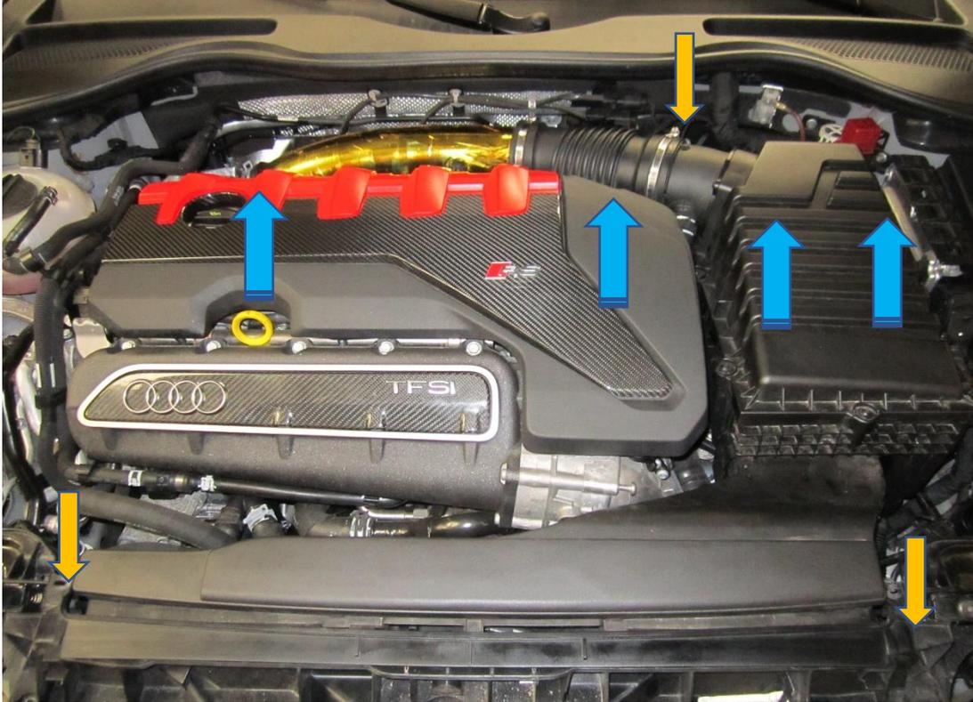
2. Unplug the MAP sensor, TPS sensor and undo the T30 torx fastener that holds the engine cover bracket and the stock dump valve. Then undo the hose clamp that holds the boost hose to the cast elbow.
