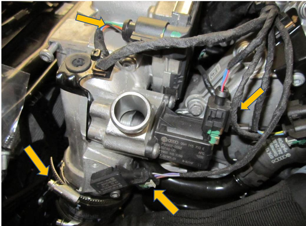
3. Remove three of the four T30 torx fasteners that hold the cast elbow to the throttle body and inlet manifold, using a 10mm socket under the five bolts that hold the inlet manifold together.
