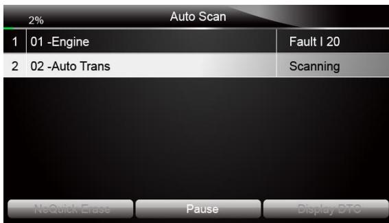
Figure 4-10 Sample Automatic System Scan Screen
