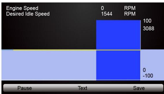
Figure 4-26 Sample Merged PID Plots Screen
