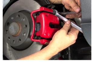
Repeat this step on the lower caliper attachment.
