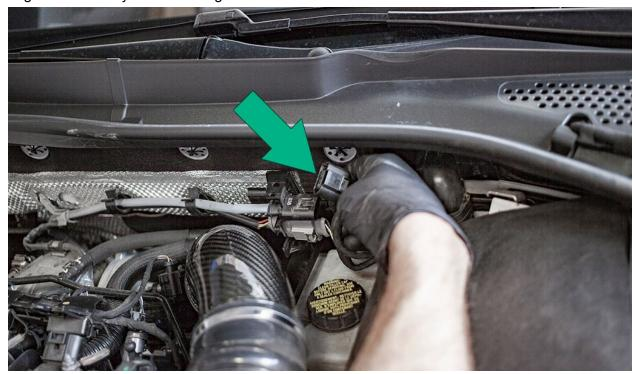
Carefully unclip the 02 sensor harness from the firewall clips and safely lay it out of the way.
