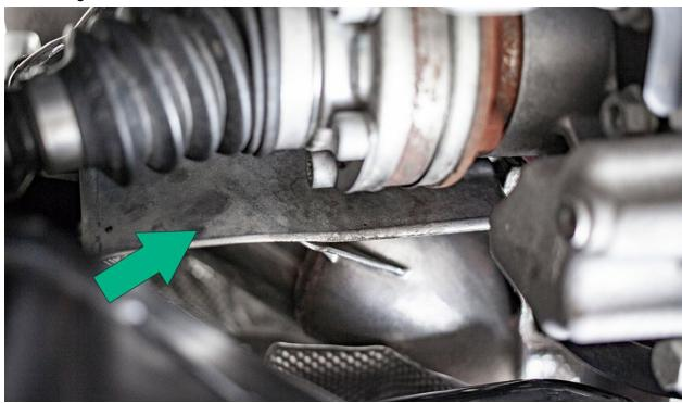
Rotate driveshaft and reinstall all three 10mm 12 point bolts.
