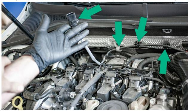
Using a 6mm allen bit, remove the factory v band clamp bolt and v band clamp. *Keep bolt & clamp for reinstallation.*
