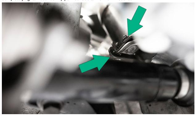
Reinstall the 02 sensor harness back into the clips and reconnect to vehicle harness clip .
