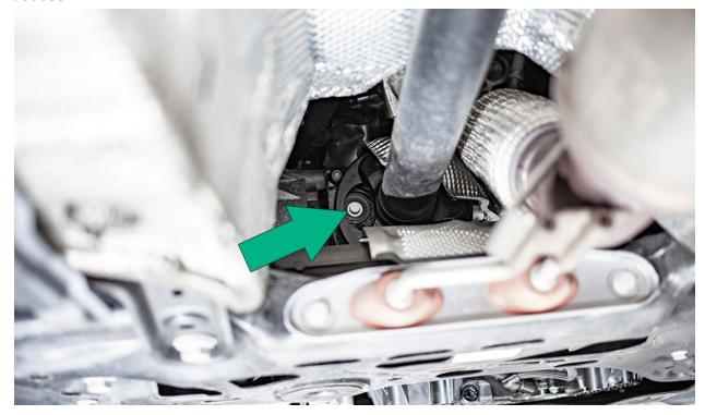
Remove both transmission mount bolts with a 16mm to allow engine movement for removal/install of downpipes.
