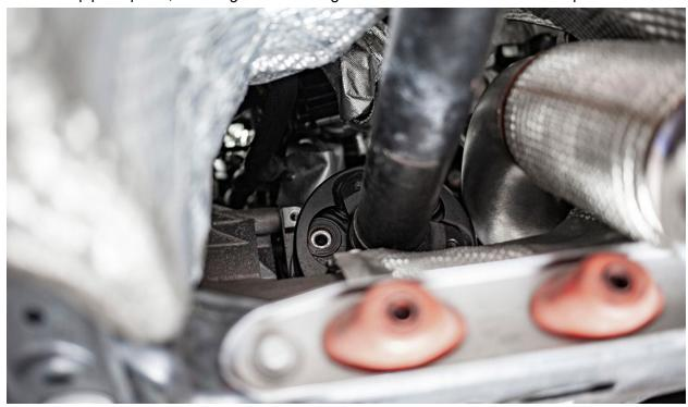
Reinstall diff heatshield, 10mm triple square bolt and 16mm nut .
