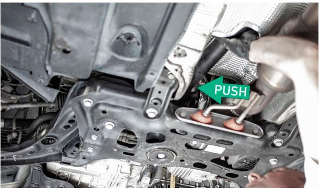
Using a 13mm socket remove the rear nut and loosen the upper nut from the downpipe support bracket located above the right side axle.
