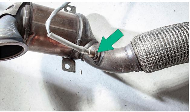
Reinstall 02 sensor into the new IE downpipe with a 22mm wrench or 02 sensor socket.
