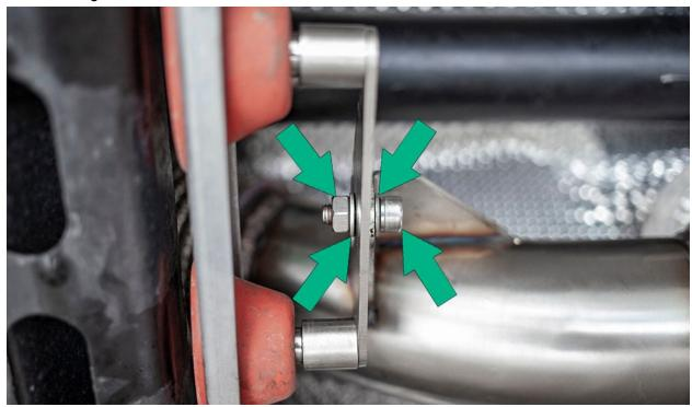
Install the mid-pipe section to the catback with included exhaust clamps. Install into place between the downpipe and catback. Adjust so that everything sits even, seated, and without binding or drooping. *Do not tighten clamps in this step.*
