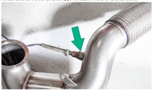
Carefully rotate the new IE downpipe into place and seat against the turbo flange.
