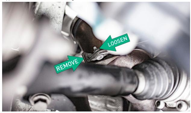
Loosen both catback exhaust clamp nuts with 13mm socket.
