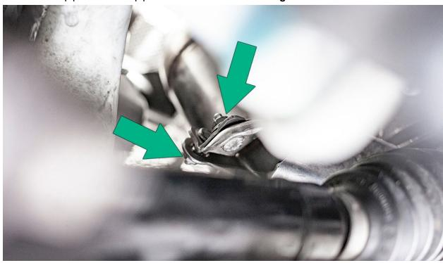
Seat IE downpipe mount bracket hangers into the factory grommets. Bracket should sit behind the downpipe bracket as seen below.
