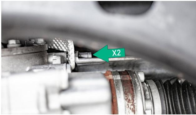
With both allen bolts removed, remove the right axle heatshield from vehicle.
