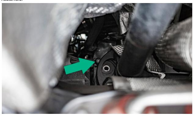
Remove both right axle heatshield bolts with 8mm allen bit. (These bolts are very difficult to see for removal, use your hand to trace the edge of the heatshield to find both bolts for removal)
