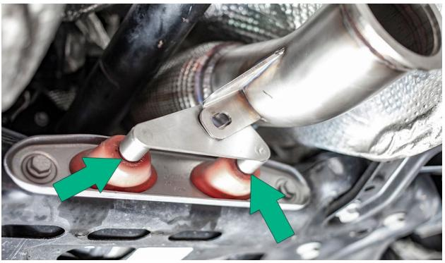
Install and tighten the included allen bolt, washers, and nut as seen below.
