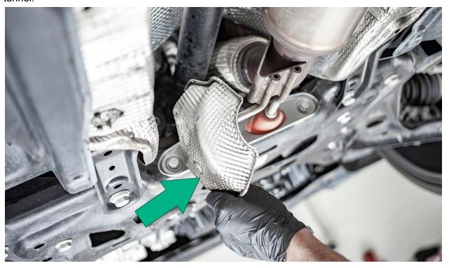
Using a crowbar for leverage, rock the engine forward and push the driveshaft out of the way of the downpipe.
