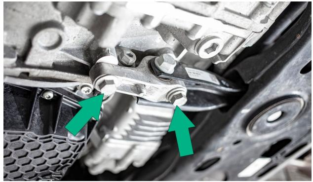
Using a 10mm triple square socket, remove the bolt from the left side of the differential heatshield.
