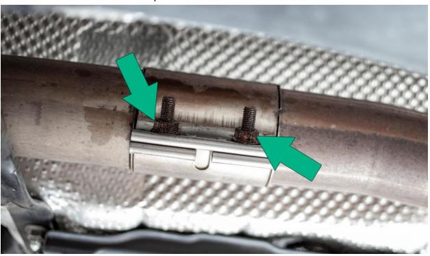
Disconnect downpipe from catback and remove exhaust band clamp.
