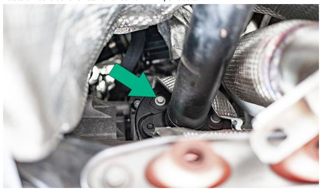
Slide IE downpipe over downpipe mount bracket and **hand tighten** both 13mm nuts.
