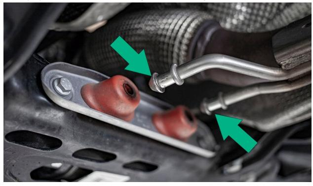
Carefully pull the downpipe away from the turbo charger then slowly rotate counter-clockwise while pulling down to remove from vehicle.
