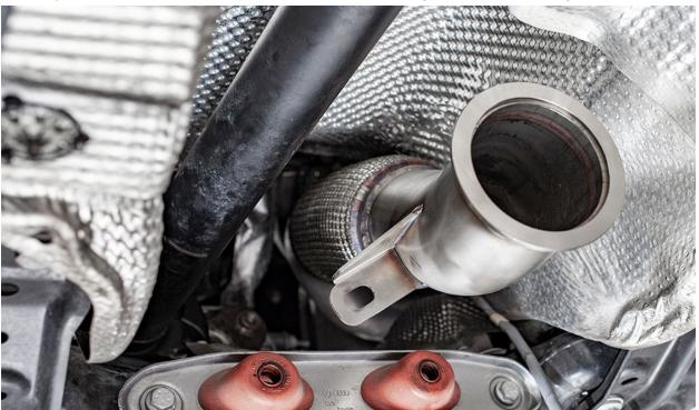
Install factory v band clamp and bolt to the IE downpipe and turbocharger. *Hand tighten bolt only.*
