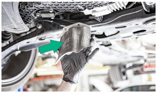
With heatshield out of the way, remove the remaining diff heatshield nut with a 16mm socket.
