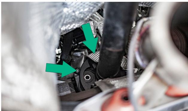
Reinstall right axle heatshield with both 8mm allen bolts.
