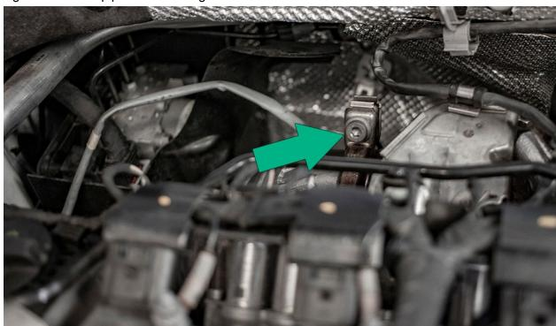
Completely tighten both downpipe mount bolts with 13mm socket.
