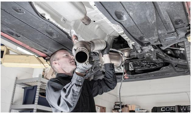
Using a 22mm wrench or 02 sensor socket, remove the 02 sensor from the factory downpipe.
