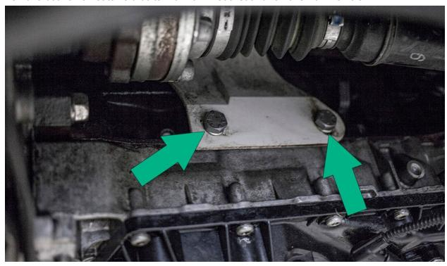
Remove both downpipe mount bracket nuts with 13mm socket.
