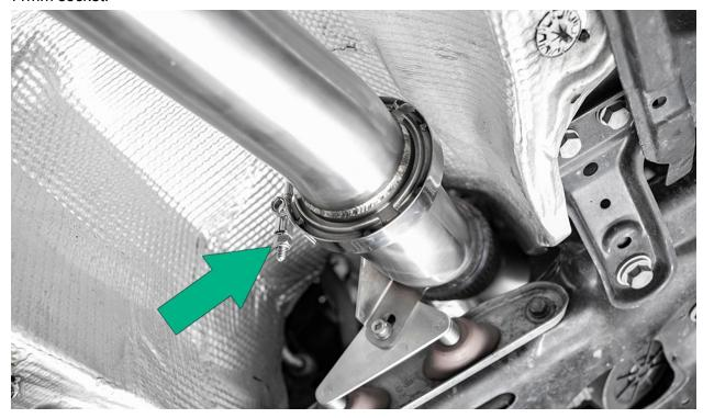
Double check that the midpipe and slip fit is properly aligned, then tighten both exhaust clamps with 15mm socket. *Note: Exhaust clamps need to be very tight, they warp to fully seal the slip-fit adapters. We recommend using an impact to completely seat them.*
