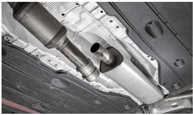
Remove both bolts from downpipe grommet mount with 13mm socket.
