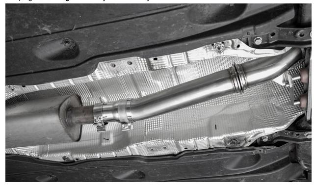
Install the supplied v-band clamp to the downpipe and midpipe flanges. Tighten firmly with an 11mm socket.
