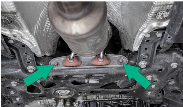
Carefully pull the downpipe away from the turbo charger then slowly rotate counter-clockwise while pulling down to remove from vehicle.
