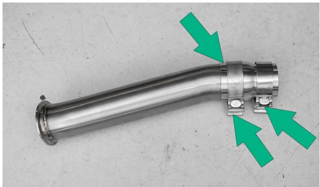
Install the slip fit section to the catback with included exhaust clamps. Install into place between the downpipe and catback. Adjust so that everything sits even, seated, and without binding or drooping. **Do not tighten clamps in this step**.
