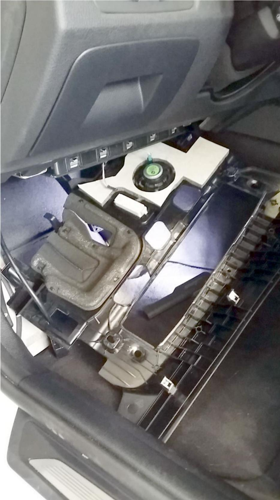
Using a long screwdriver push in on the rubber firewall cap pushing it in to the interior compartment. You'll see it fall down by the pedals and can put it away for safe keeping. Feed the OBDII wire from the interior through the hole to the engine compartment. Note this is also a great place to route your BMS DATA cable if equipped.
