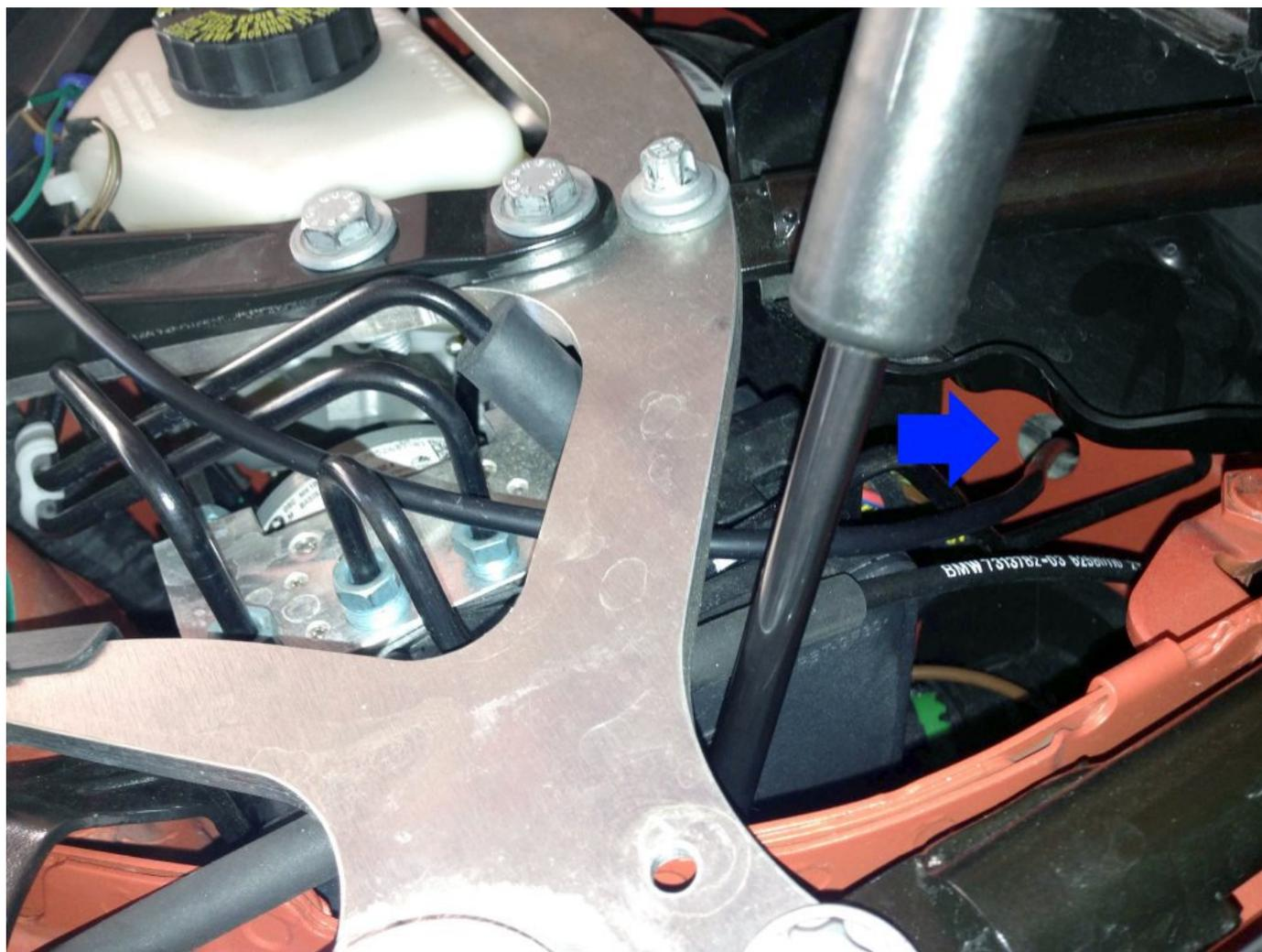
Plug the OBDII wire in to the JB4 green/brown molex connector.
