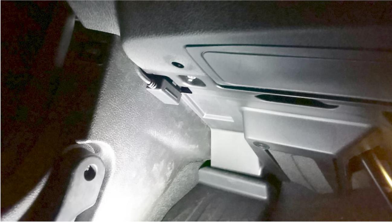
6) Tuck the now fully installed JB4 control box out of the way as shown. The wiring harness should be routed under the rubber cowl seal for a clean fit once the cowl cover is reinstalled. Tuck extra wire length out of the way taking some care to ensure nothing is too close to the moving mechanical parts of the windshield wiper arm/assembly.
