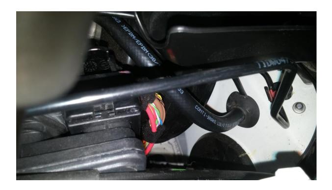
Connect the OBDII cable to the JB4 harness by plugging in the connector.
