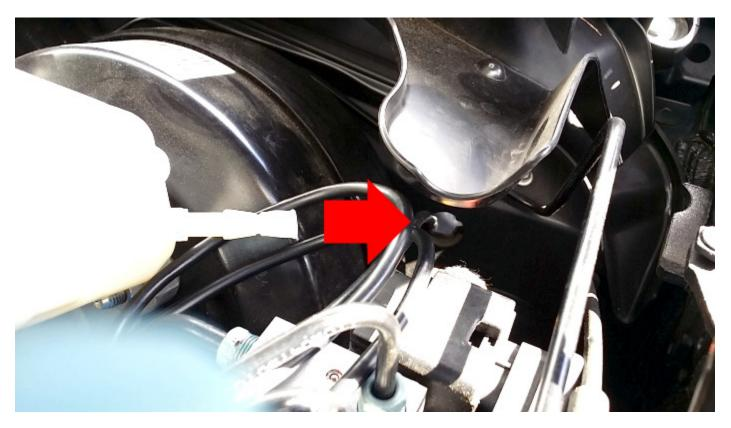
Note those with a manual transmission have the clutch line run through this same hole. You'll need use a coat hanger to pull CANbus wire around the grommet. Alternatively you can use cut a small slide in the grommet to facilitate feeding the CANbus wire through.
