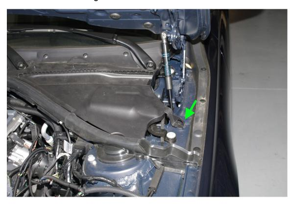
Pull up on the ring and pull the plastic cover forward to remove.
