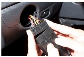
Step 3: thread the wire up to the OEM headlight harness. To do this you must first take off the plastic fuse cover under the Headlight switch. This cover comes off by a simple pull from the bottom up.
