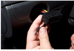
Step 5: On the sides of the wiring harness connector, you will see number labels. Those labels mark the Pin number for each slot. The pin number to activate the front fog lights is pin #8. Your connector should look like the picture on the right when installed properly.
