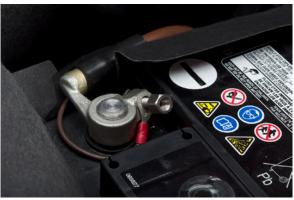
After tightening the nut, proceed to secure the brown harness wire to OEM wire that connects to the negative terminal. Use a zip tie and secure it about three inches away from the 90 degree kink in the brown OEM wire.
