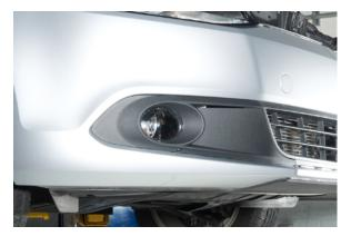
Now reinstall the top grille by pushing the bottom clips in, and then reinstalling the four screws at the top. Use your T25 torx driver to ensure the grille is secure.
