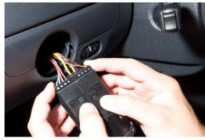
While pushing the clips, gently pull on the switch, backing it away from the connector.
