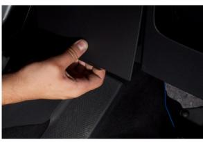
Now take the end of the wire that you have threaded through the firewall, and pull it up By the left side of the fuse box, and up to the OEM harness.
