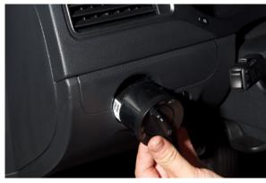
Upon reaching the proper position, the switch will snap into the dash
