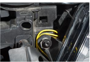
Next go around the bumper support downwards and bring the wires back up on the other side. Now the wires are tucked behind the bumper support and have a clear accessible path to the driver side and passenger side headlight.
