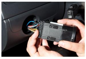
For added security, before reinstalling the switch, use a zip tie to ensure the wire is snug against the harness so it doesn't have play room.
