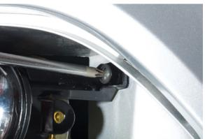
Position the fog light into the housing. Insert the side with clips first and then using a T25 torx driver, twist the screw in to secure them in place.
