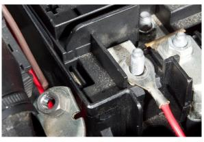
Take the red cable and reinstall the nut. Use the ratchet to tighten down the cable. Exercise caution not to over tighten the nut.
