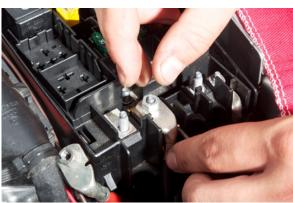
Next install the red wire from the harness positioning the loop around the terminal where the red wire sits.
