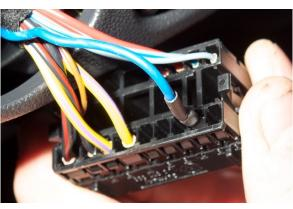
Step 5: Connect the Euro Switch to the OEM connector.
