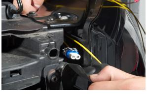
There is a rubber piece over the bolt shown to the right. Remove it and route the wires as shown.
