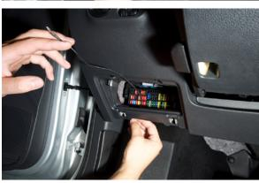
After routing by the fuse box you can put the cover back on.
