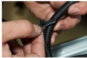
The finished product should look threaded like the picture on the right. After threading the wire through, you can reuse the OEM tape and re tape the clips. After repeating this for all of the clips, reinstall the clips in the trunk arm.
