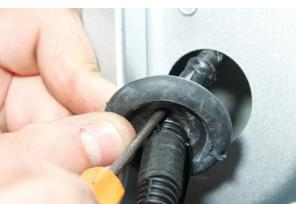
After making the incision, pull the two wires from the harness through so it sits inside of the trunk lid.
