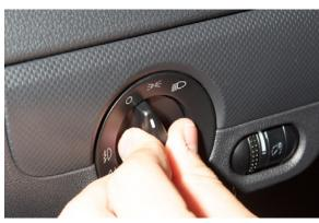
At this point the headlight switch will pull out easily. Be cautious pulling the switch out, as you do not want to damage the harness that connects to it.
