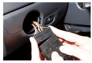
Once the switch is out, you will notice numbers on the sides of the harness plug. The pin you want to connect the wire to is pin #9.
