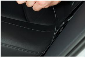
To release the seat, go to the trunk and pull on the switch shown to the right. It will be easily visible once you pop the trunk, and is located on the driver side.
