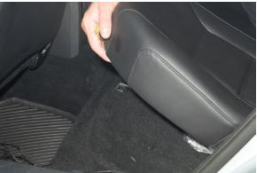
Make sure the latch towards the rear of the seat releases as well.
