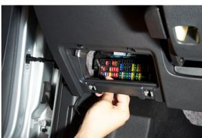
Continue routing the wire up through the headlight switch hole.
