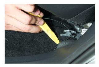
Once you have gotten this far, it's time to release the seat, and flip it down to allow you to tuck the wire towards the trunk.
