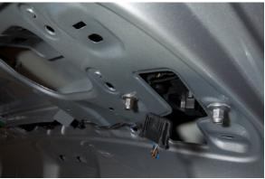
Next, take a trim tool and unhook the clips that run up the arm of the trunk lid. Remove the clips.
