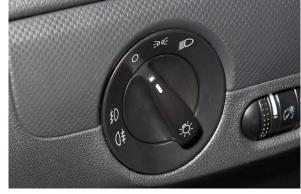
To remove it, Push in on the button, and twist the switch about 15 degrees clockwise.
