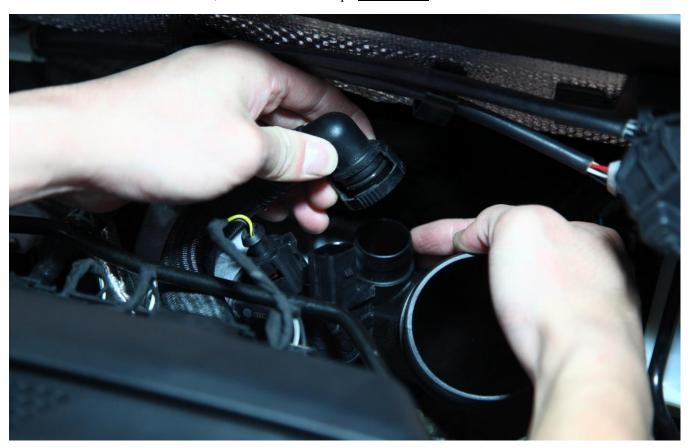
Step 5- Remove 3 5mm Allen Bolts on BOV using 5mm Allen wrench and Snake Magnet (recommended)
