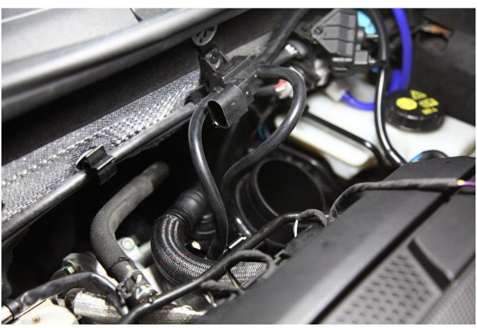
Step 19- Use WD40 to lubricate inside of silicon hose and connect 14cm piece to BOV
