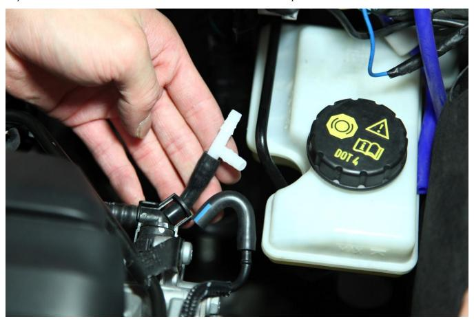
Step 6- Using Dykes (cutting pliers) cut piece of silicon hose (measure off engine cover or approx 30-33cm)
