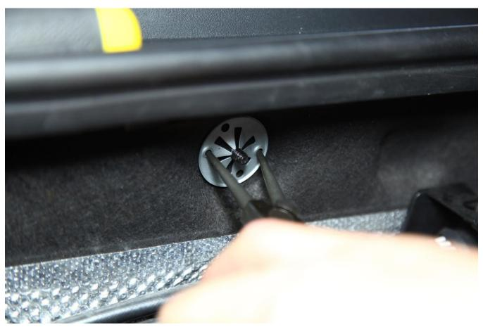
Step 11- Using snap ring pliers, attach Control Solenoid and bracket to firewall (connector facing vehicle right)
