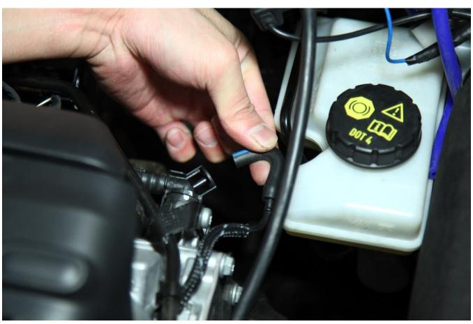
Step 5- Use WD40 to lubricate inside of silicon hose and connect 4cm piece to "T" connector
