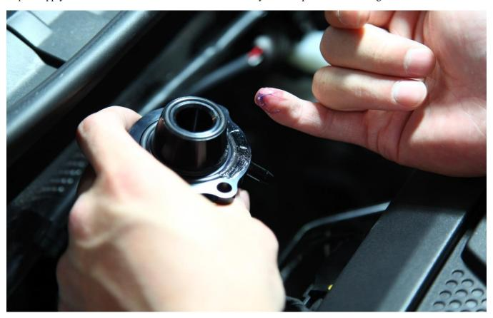
Step 2- Install BOV with 3 Allen Bolts (careful not to cross thread), and make finger tight (approx. 12ft/lbs)
