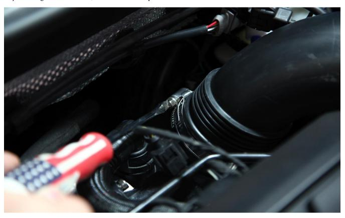
Step 2- Using Channel lock pliers, remove pinch clamp on front of intake hose
