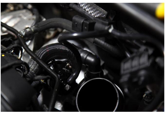
Step 17- Using Dykes (cutting pliers) cut piece of silicon hose (measure off engine cover or approx 14cm)
