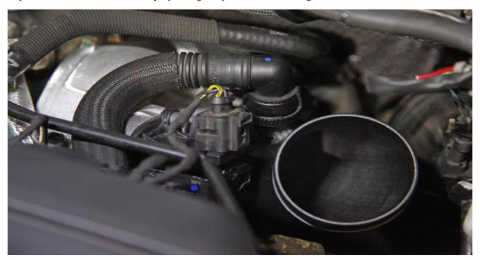
Step 3- Remove T25 Torx bolt from Turbo housing
