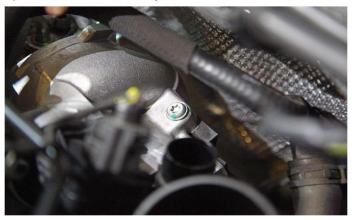
Step 4- Remove TIP by rotating towards firewall then slide towards left side of car
