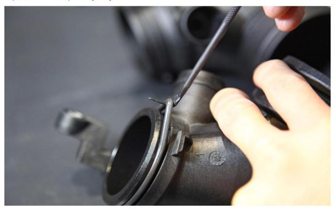
Step 6- Place O-ring onto Leyo TIP
