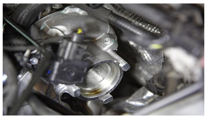
Step 5- Remove factory O-Ring using small screwdriver (dentist tool)
