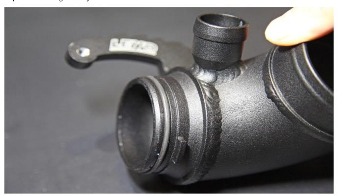
Step 7- Install Leyo TIP back into Turbo housing and tighten T25 Torx bolt
