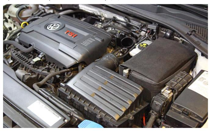
Step 2- Remove PVC hose on TIP by squeezing and plastic tabs and lifting
