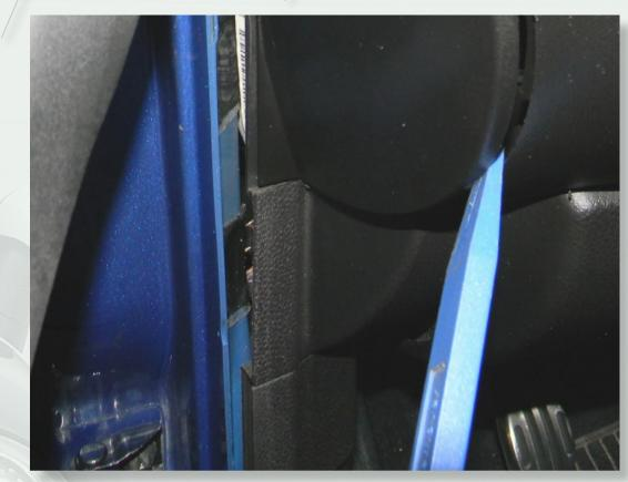
Gently feed the flat wiring harness from the display unit behind the rubber seal, through to the opening in the left hand side of the dash.
