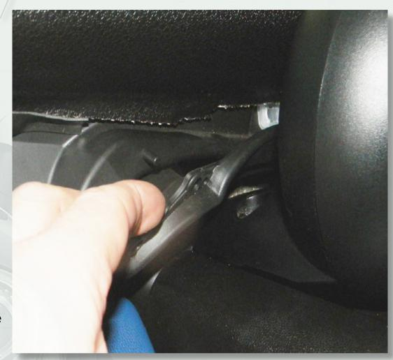
Pull the rubber seal located above the steering column forward.
