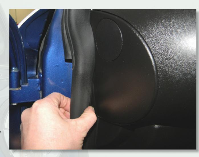
Pull the weather strip off of the driver's door jam just enough to access the left hand dash end panel.
