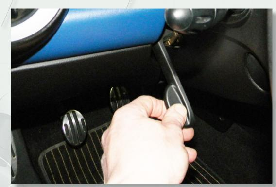
Using a plastic trim tool, release the driver's side dashboard trim piece by prying out on the bottom.
