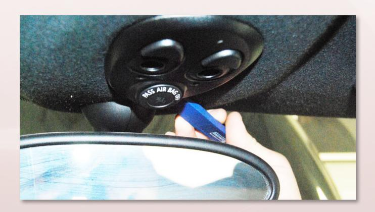
Once the bulb assembly itself is dangling in front of you, take note of two black knobs that house the bulbs. Twist the knob to the left 1/4 turn and the bulb will back out easily. Holding the black tab in one hand, pull outwards while slightly wiggling the bulb. The bulb is strong and will not break when pulling hard on it. Once the bulb is removed, slide the Front Dome LED into the bracket where the incandecent bulb sat - this may take moderate effort.
