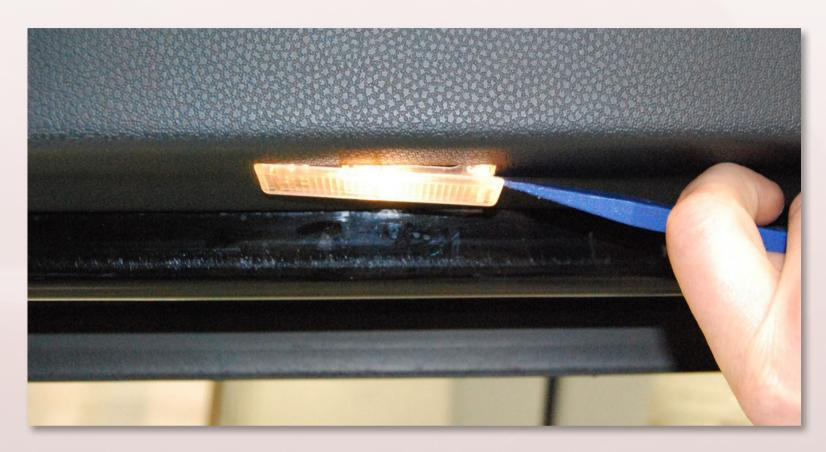
The bulb housing will slide out of the door and dangle with its connector clip. Carefully, using a tool if the bulb is hot or hard to access, pry out the existing bulb. Replace with the T10 Door LED. Repeat on opposite side.
