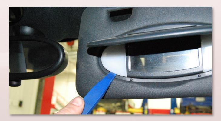
Using moderate force, pull out the incandecent bulb from its housing. Extra effort may be required for your particular vehicle. Once the bulb is removed, take the Sun Visor LED and insert it into the flat tabs, securing it against the base of the housing. These lights are polar sensitive; test the function of the light - if it does not illuminate while the adjacent bulb does, simply remove the bulb and rotate it 180 degress and reinsert.
