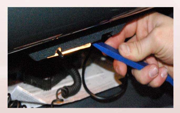
Replace with the 36mm Festoon LED and resinstall the housing.
