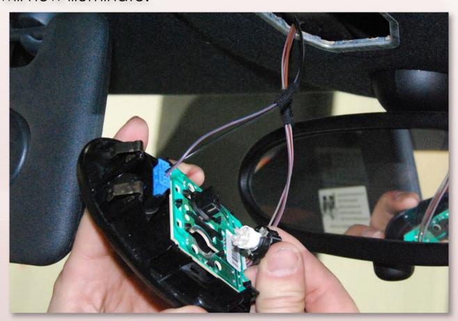
Press back into place the front map light housing. Then press the new, LED-lit bulb housing back into its original place.
