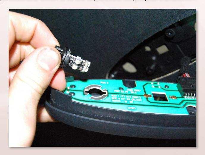
After removing the existing bulbs, carefully insert two T10 Base Cool White 8 Chips and replace the center incandecent bulb with the 36mm Festoon. The procedure for checking for correct polarity is the same for the other LED's - insert the light, check for illumination (making sure electricity is being supplied) and rotate the LED if necessary.
