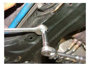
After installing all 7 rivets you can bolt the forward brackets to the frame using the (4) 17mm bolts.
