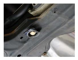
Before installing the plate, slide the rubber bushings onto the skid plate.
