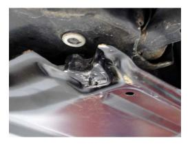
To install the skid plate you first need to slide the rear of the plate into the rear brackets and then install the front two bolts. (Having an extra set of hands would be very helpful.) Tighten all 5 bolts holding the skid plate in place at this point and you are finished.
