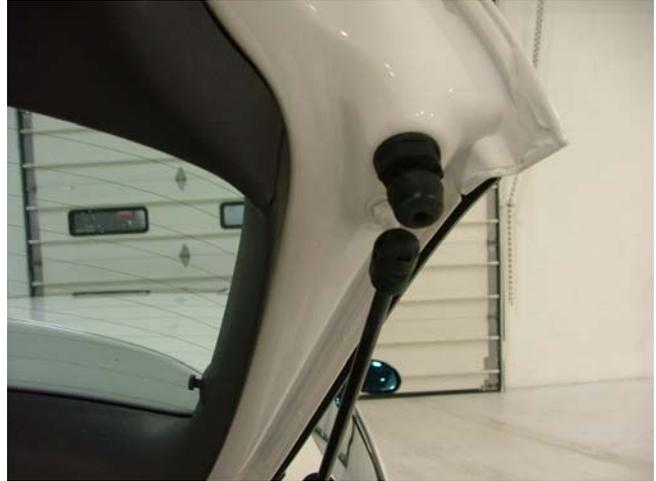
Then use a 13mm wrench to remove the old mounting pin. Install the new mounting pin and the new hatch strut. Repeat for the other side.
