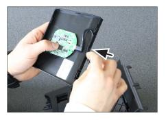
Connect the USB connection cable to the board on the bottom of the Inbay tray. Route the cable through the existing opening as shown.
