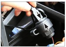
Connect the InBay USB connector to the USB socket of the voltage transformer
