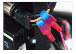
Caution - Before connecting the voltage transformer, check the correct polarity with a voltmeter!
