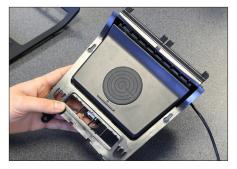
Install the Inbay storage on the OEM storage unit and rebuild it all previously dismantled parts again.
