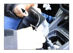
Pull the gear shift cover over the shift knob
