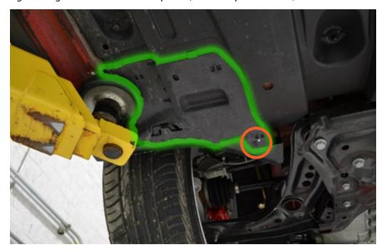
**2.** We need to remove this panel in order to install the adapter. To do this, simply push in on the locking tabs (circled in photo below), while simultaneously sliding the panel toward the rear of the vehicle.
