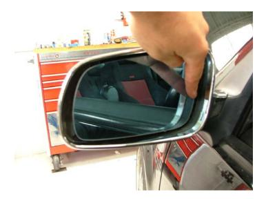
Use fingers to get behind mirror assembly on the outside portion of mirror (See picture), now by applying GENTLE force towards mirror assembly the mirror should "pop" out of its holding mechanism, make sure to apply pressure closest to the center of the mirror to prevent damage to mirror.
