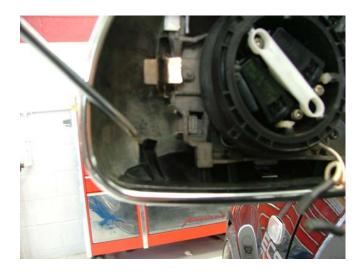
Make sure to reattach heated mirror wires (If equipped) to their original locations. When reattaching mirror lens to mirror assembly make sure to use the palm of your hand to apply even pressure to attach lens to clips, GENTLY push until mirror "clicks" in place. (See picture)
