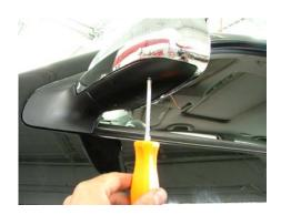
Gently pull up on mirror cap until cap is out of guides. You will notice that the black trim underneath mirror cap is still attached, unclip black trim from mirror cap and set both pieces aside until reinstallation. (See picture)
