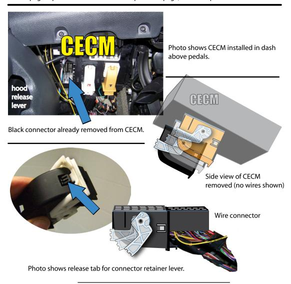
Next, we'll show you how to split the two halves of the wire connector to install the yellow wire we attached to the Euroswitch in Step 4.
