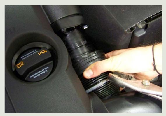
Using a T20 Torx, remove the two screws that hold the intake piping to the intake scoop.
