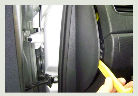
Route the blue wire up into the void behind the headlight switch.
