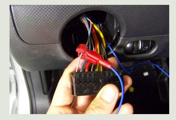
Tidy up and secure the harness wires. Reinstall the headlight switch, fuse box cover, and underdash panel.
