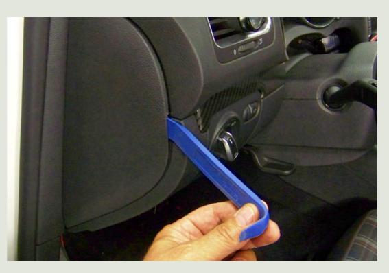
Use the trim removal tool to pry the upper dashboard trim free, then pivot the entire piece out of the dash.
