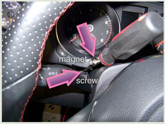
Remove the three screws from the lower edge of the underdash panels.
