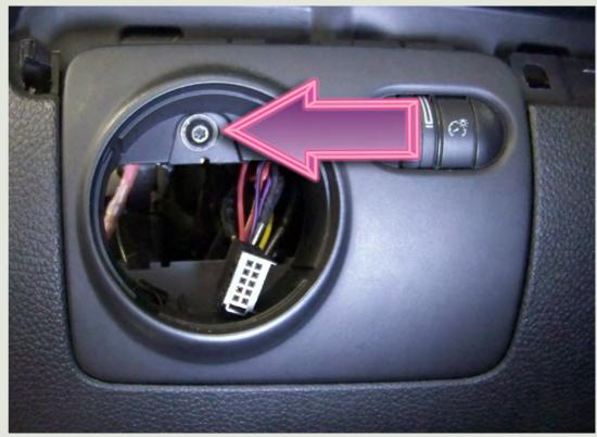
Remove the dash light dimmer rheostat. Squeeze the two plastic tabs (arrows) to release the snap clips, then pull the dimmer straight out, connector and all.
