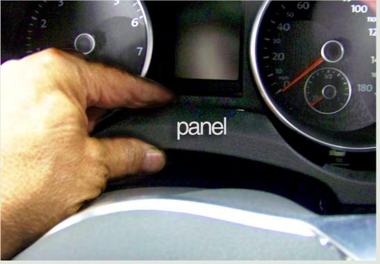
**Service Tip:** The trim panel is attached to a leatherette cover flap. Lift the trim piece far enough to expose the screw (arrow) at the top of the dash panel.
