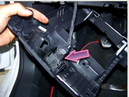
Install the new dash panel onto the dashboard frame.
