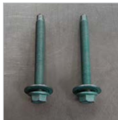
2 Rear Subframe Bolts M12 x 1.5 x 110
