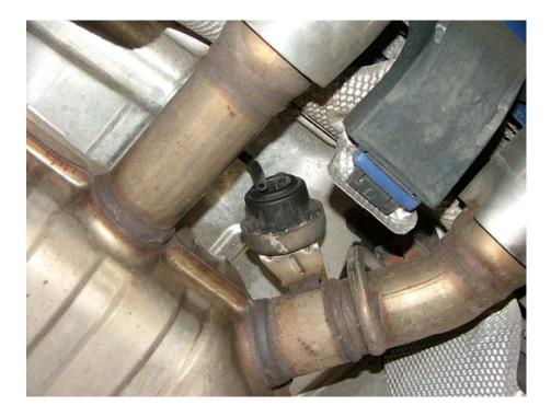
Using a pry bar to release the hangers, remove the exhaust out from under the car.
