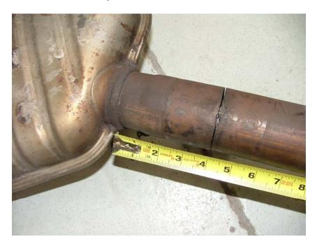
**Final Step:** Reinstall the back half of the exhaust; make sure to reconnect the vacuum line. Using the supplied clamp install the resonator delete pipe in place of the stock resonator, tighten both clamps and make sure that the exhaust does not come in contact with the drive shaft or anything else. After that reinstall the cross brace that was removed earlier and the installation is complete.
