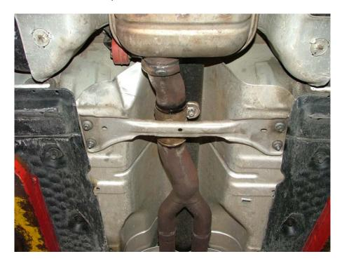
Then loosen the 13mm nuts on the exhaust clamp.
