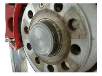
Be sure to remove any dirt or grime from the face of the rotor and the back of the wheel to insure a clean mating surface.
