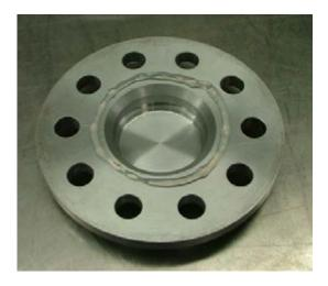
Apply a small bead of the supplied silicone sealant to the back of the new spacer. This will eliminate the possibility of dirt or water getting into the wheel bearing and causing it to fail prematurely.
