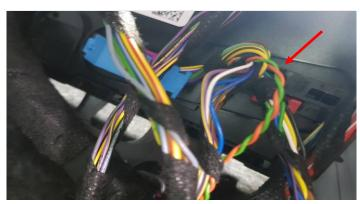
The Can ends in the blue connector socket of the ecu.
