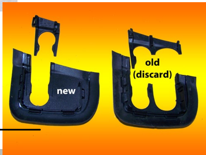
Water tray original retainer and replacement blockoff.
