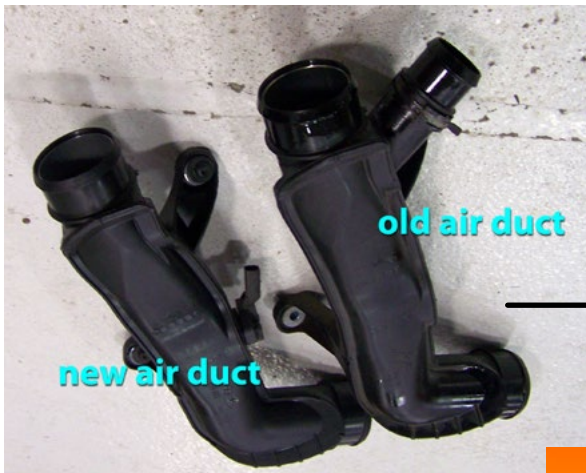
Old and new air ducts, side by side.
