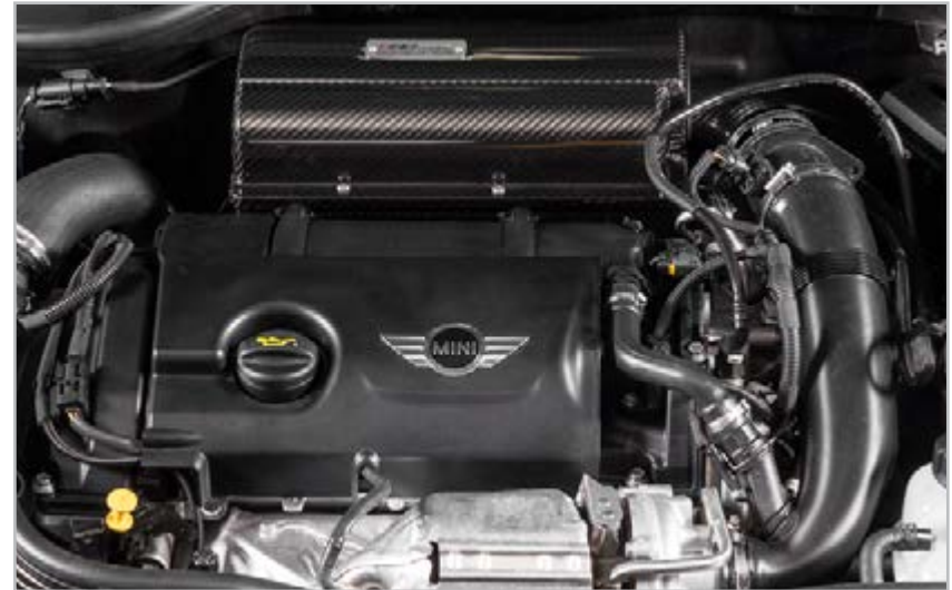
MINI Cooper N18 Engine Identified by the full cover.
