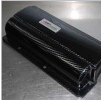
Upper Intake Box
