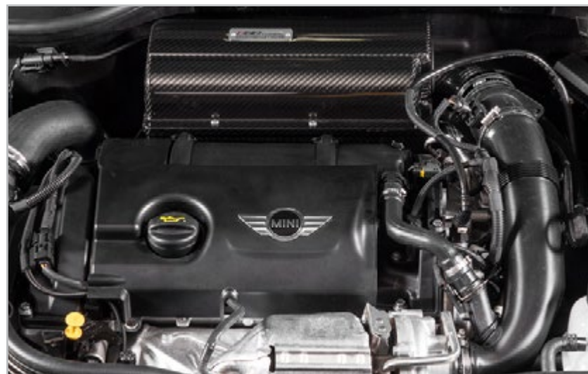
MINI Cooper N18 Engine Identified by the full cover.
