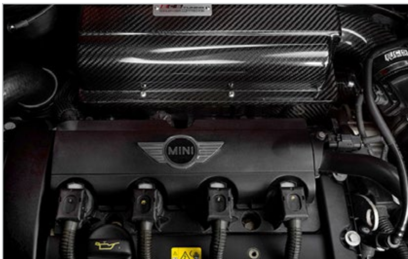
MINI Cooper N14 Engine Identified by the visible coil wiring harnesses.
