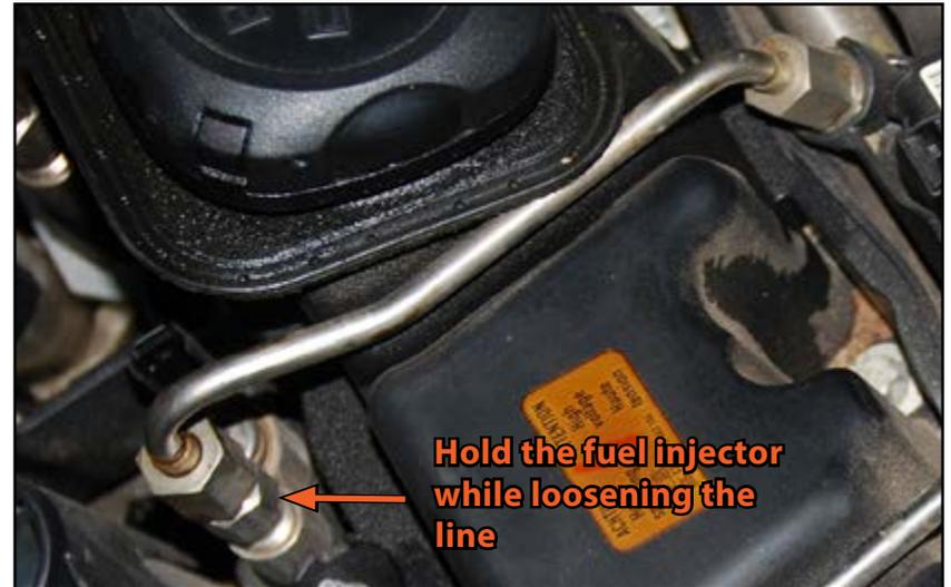
**Hold the fuel injector while loosening the line**
