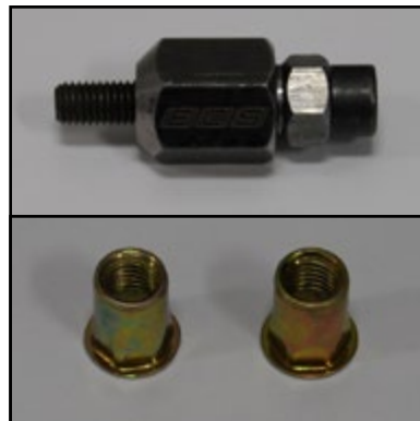
Riv-Nut Installation Tool and Riv-Nuts (2)
