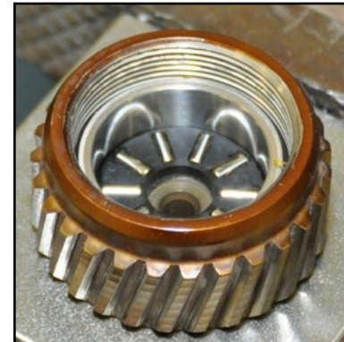
Install one bearing
