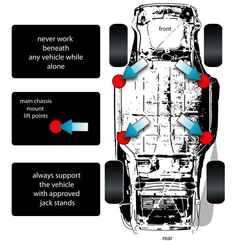
Improperly lifting the vehicle can result in personal injury and vehicle damage.
